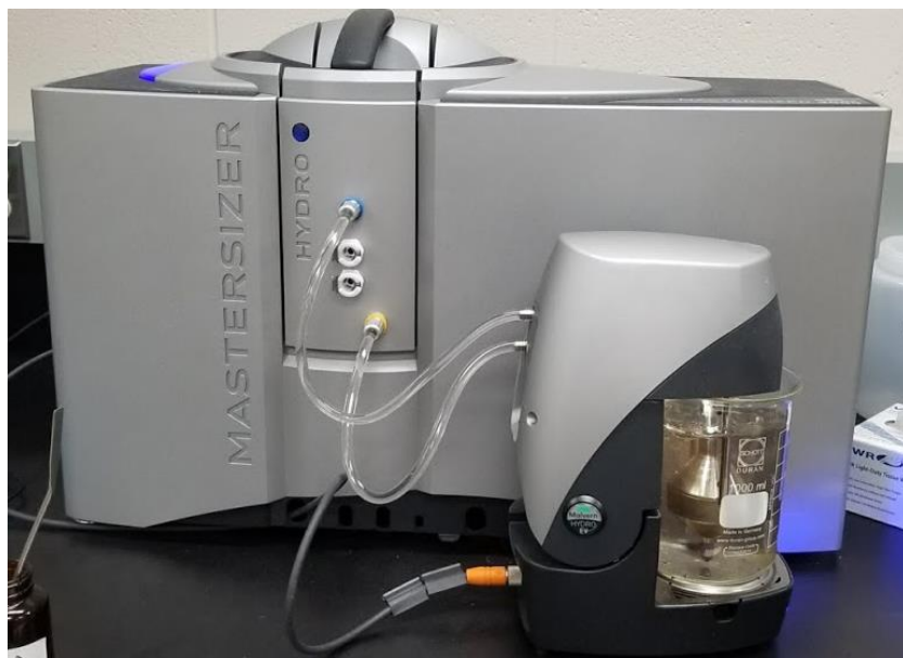
Fig 3.1. The Malvern Mastersizer 3000 used for determination of biosorbent particle size.
