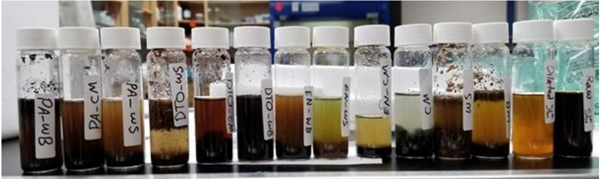
Fig 3.12. All biosorbent and pregnant leach solution mixtures with diluted and undiluted leach solutions. Operation conditions: 1 g biosorbent and 20 mL diluted PLS mixture after shaking for 24 h at room temperature and 48 h of settling.
