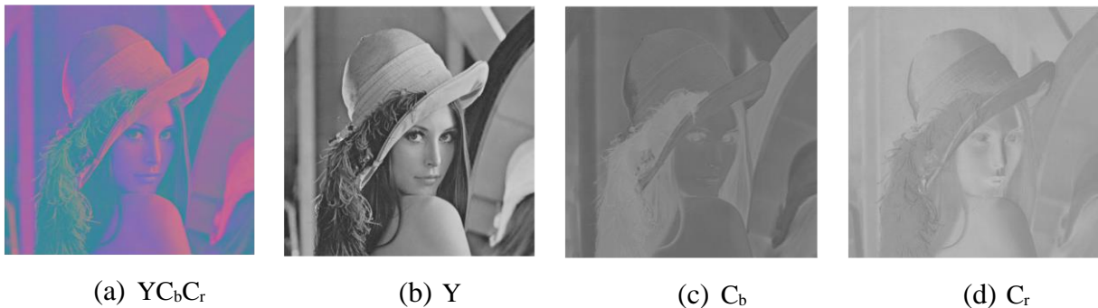
Figure 2-4: YC_bC_r color image (a) and Y, C_b , and C_r components in (b), (c), and (d) respectively.
