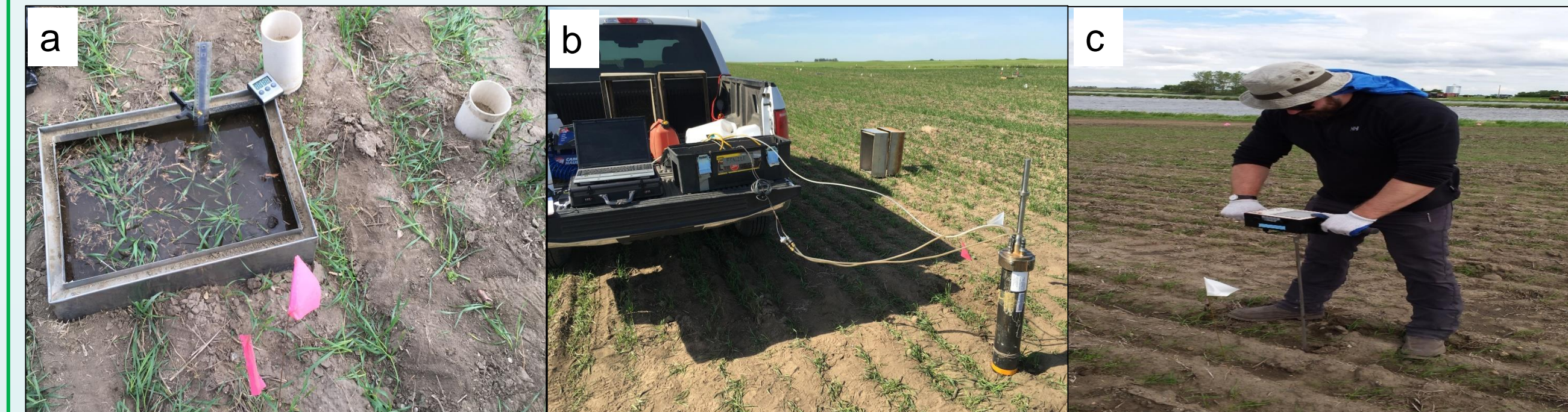
Fig. 2. Hydraulic conductivity (a), air permeability (b) and soil resistance (c) measurements in compacted and subsoiled treatment plots at the North Central Butte (NCB) Solonetzic site in June 2016.
