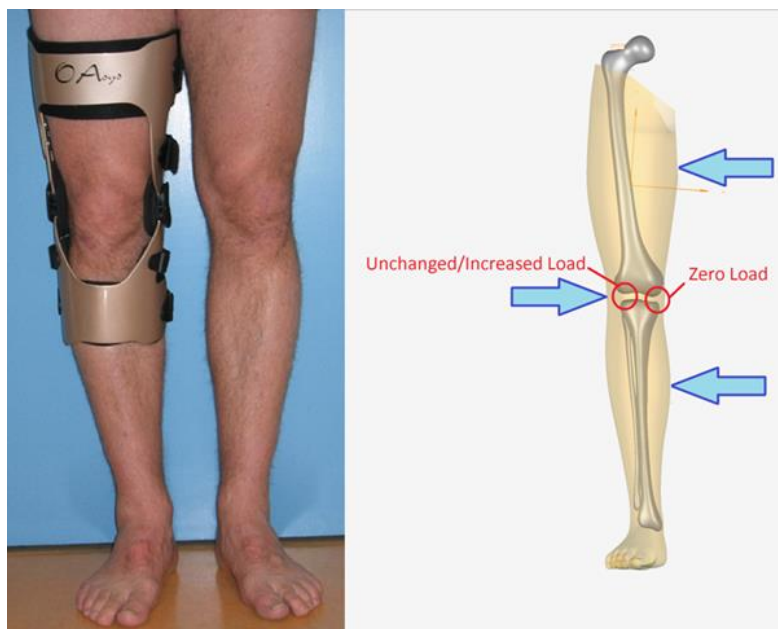
Figure 2.4: Left: An example of a knee brace, reused with permission 16 . Right: A diagram showing the moment-generating loads applied by a knee brace
