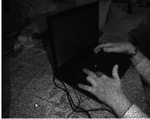
Figure 3.4: Kinect's infrared structured light captured by its infrared light sensor
