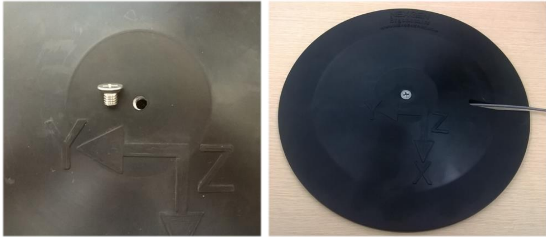
Figure 5. Mounting screw for the accelerometer through the top of the rubberized seat pad.
