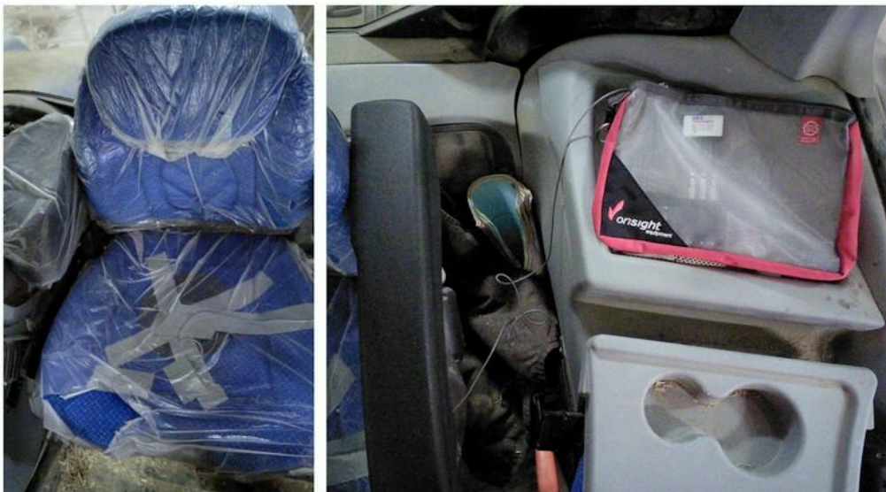
Figure 15. Place the DataLOG in the Pelican Case (or if there is insufficient space, the Onsight Pouch), and secure the case inside the vehicle cab.
