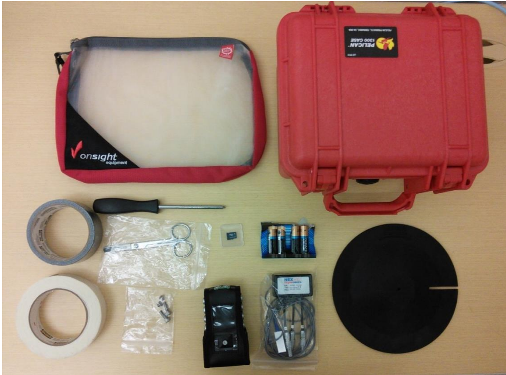
Figure 8. Equipment for measuring WBV. Measurement equipment and supplies are to be stored and transported in a pelican case and onsite equipment bag.
