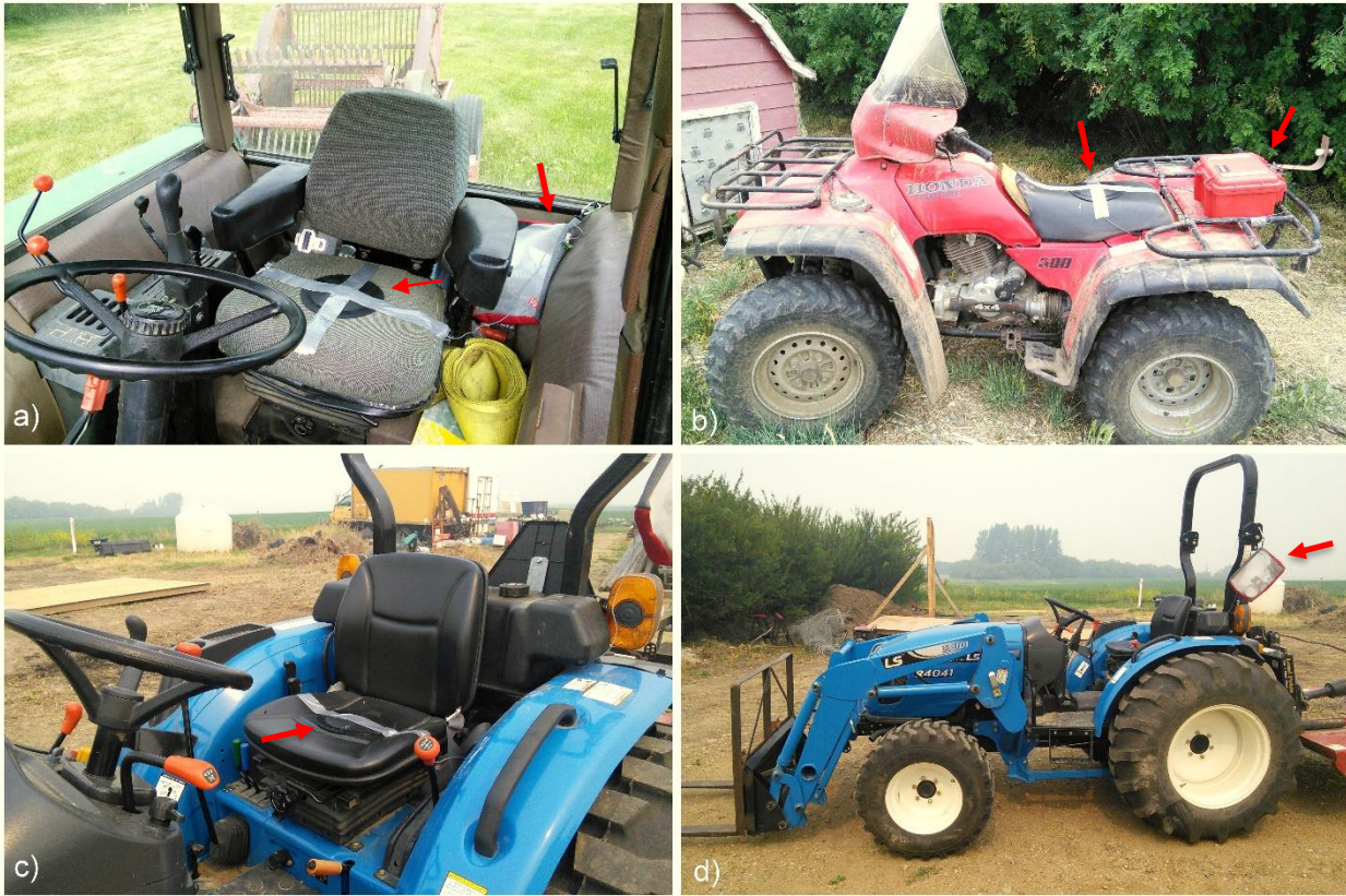
Figure 3. Different whole body vibration onsite measurement cases. Figure a) the whole body vibration measurement on the seat inside a tractor cab: the seat pad set up on the surface (arrow) and data recorder safely stored in the onsite pouch behind it (arrow); Figure b) the same set-up (arrow) on an all-terrain vehicle, the data recorder was stored in a pelican case (arrow); Figure c) a measurement (arrow) made on a tractor seat without a cab; Figure d) the onsite pouch (arrow) was placed closest to the seat.
