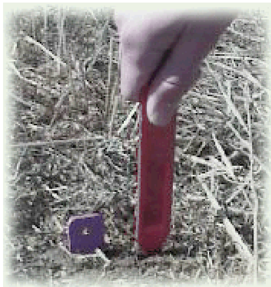
Figure 1. PRS™ Probes inserted directly into a moist field soil.
