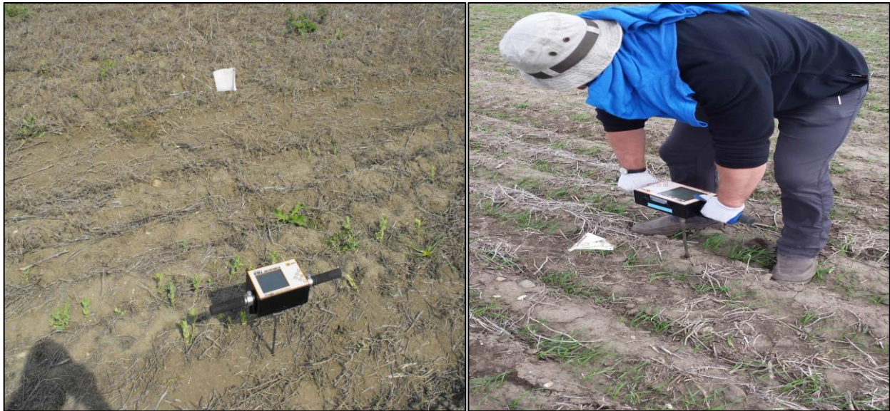
Figure 3.15. Rimik CP40-II penetrometer measuring soil resistance at South Central Butte site.
