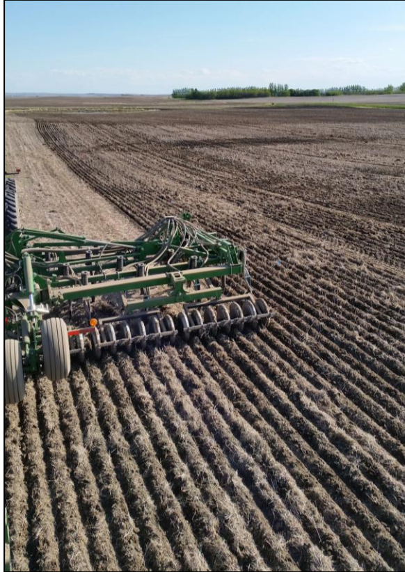
Figure 3.9. John Deere 1830 Air Hoe Drill with paired row double shoot openers used to seed plots.
