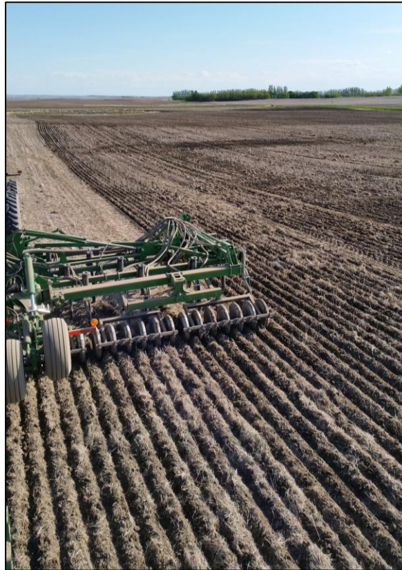
Figure 4.6. John Deere 1830 Air Hoe Drill with paired row double shoot openers used to seed and fertilize the plots at the FRM trial site.
