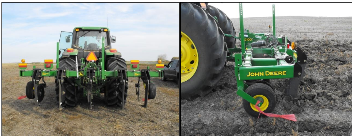
Figure 3.6. John Deere 2100 minimum tillage subsoiler mounted on John Deere 6170M tractor 3- point hitch.
