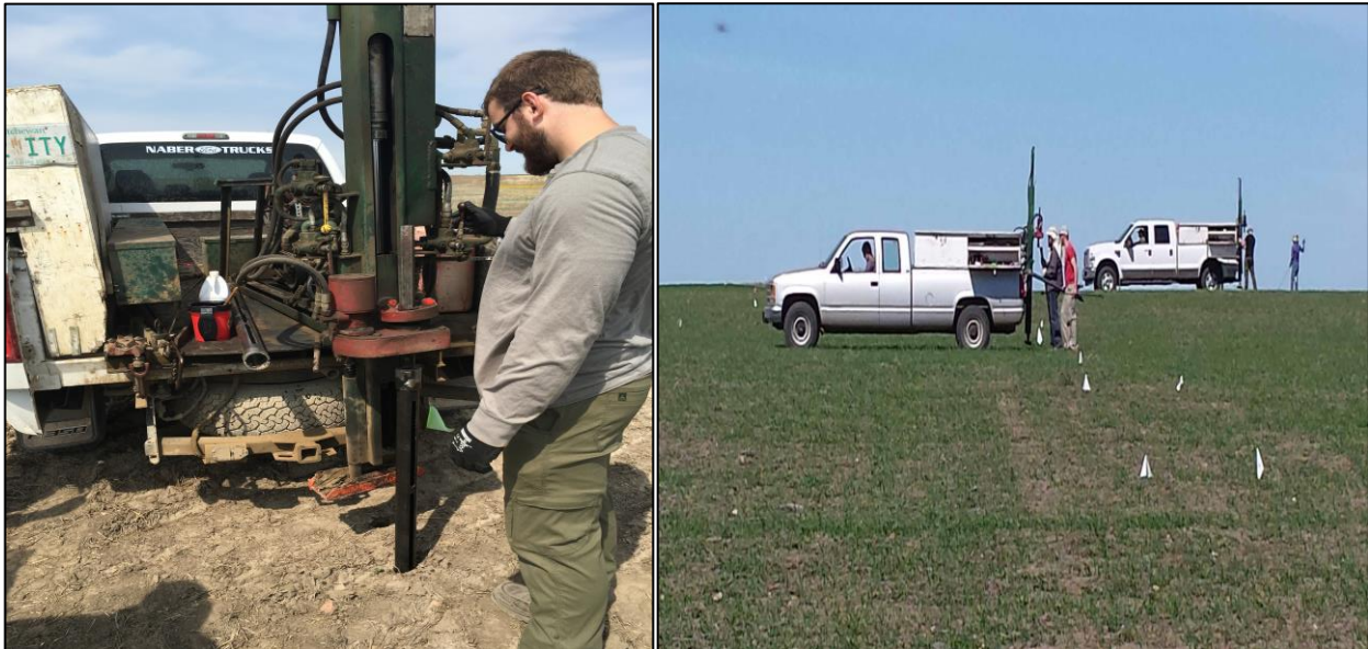
Figure 3.14. Field core sampling for bulk density and moisture using a Gidding truck mounted hydraulic punch unit.
