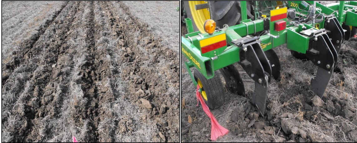
Figure 3.7. Loosened soil (left) after one pass with the John Deere 2100 minimum-till subsoiler (right) at the South-Central Butte site in October 2015.
