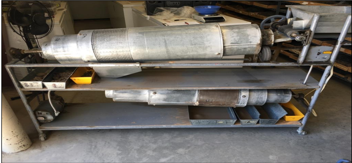
Figure 4.11. Motorized sieve machine used to determine aggregate size.
