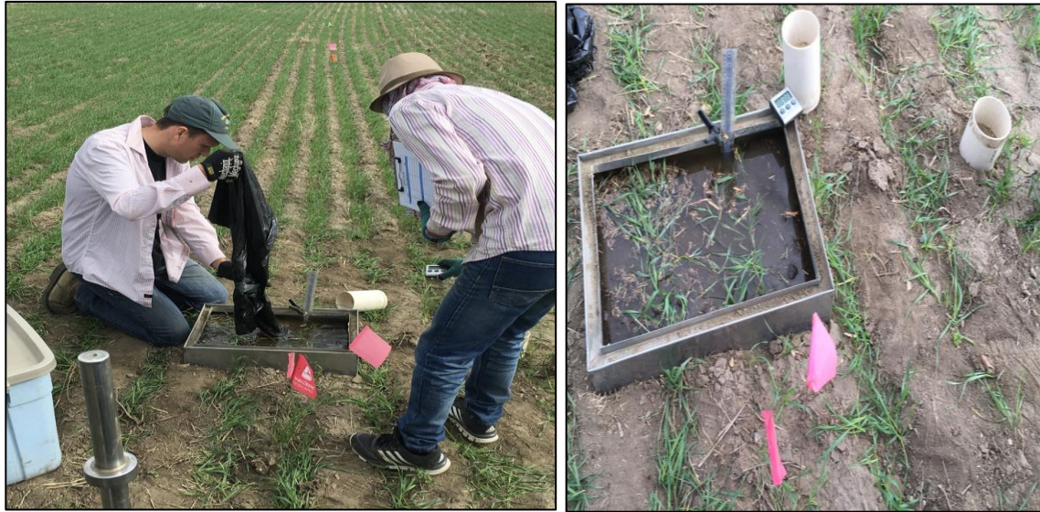
Figure 3.21. Square ring and PVC cores installed to determine hydraulic conductivity at SCB and NCB sites.
