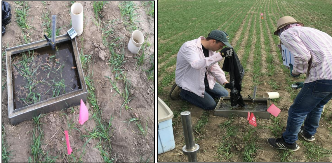
Figure 4.14. Square ring and PVC cores installed to determine hydraulic conductivity at FRM site.
