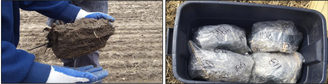
Figure 4.10. Undisturbed samples removed from the field two days after seeding for measurement of aggregate size and stability.
