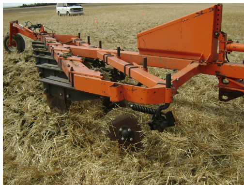
Figure 1. Non-inversion subsoil tillage implement called a Paraplow in operation
