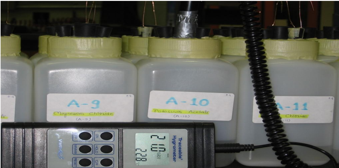
Figure 3-6: (a) Relative humidity environment created inside the lab, and (b) Relative humidity and Temperature measurement using Humidity probe.
