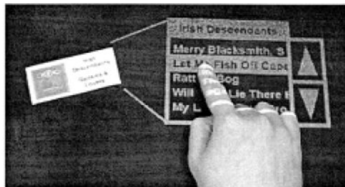
Figure 2.13 An example of live card, an interactive music selection menu is displayed upon recognizing the card [54].
