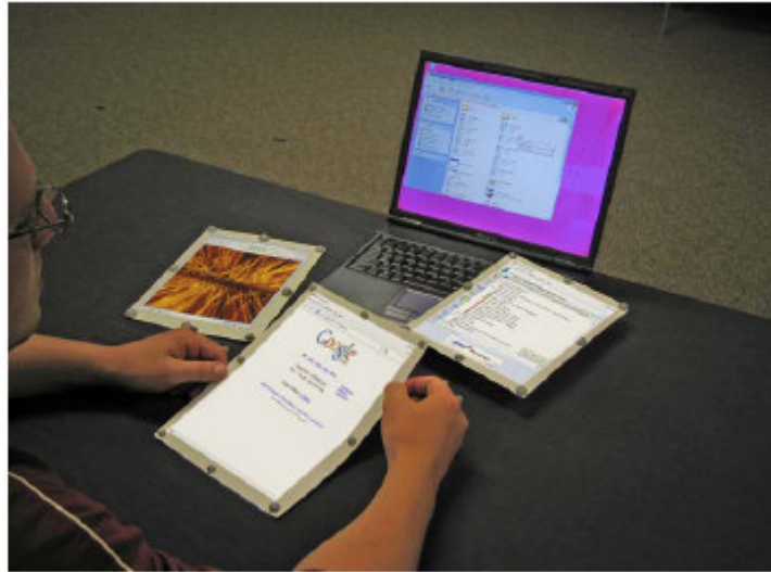
Figure 2.14 A snapshot of PaperWindows prototype in action, three pages are augmented with projected windows [28].
