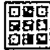
Figure 4.7 An exact image of the tag after rotation and thresholding is applied to the original sub-image.
