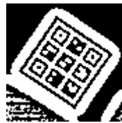
Figure 4.5 Threshold sub-image of a candidate tag. The extracted region is bigger than the tag to compensate for various rotations.
