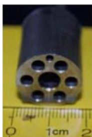
Figure 8. Six-shooter sample holder for in situ XAS data collection. The total diameter of the six shooter is 18 mm, and the diameter of each hole for the sample is 4 mm. The small hole at the top connects to the thermocouple, and the larger central hole is used for beam alignment.
