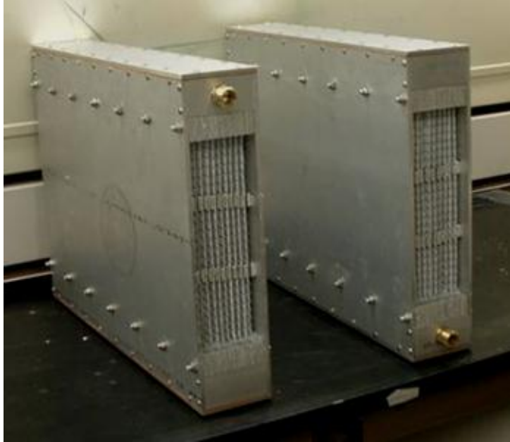
Figure 2.3: Photograph of the two fully assembled LAMEEs.
