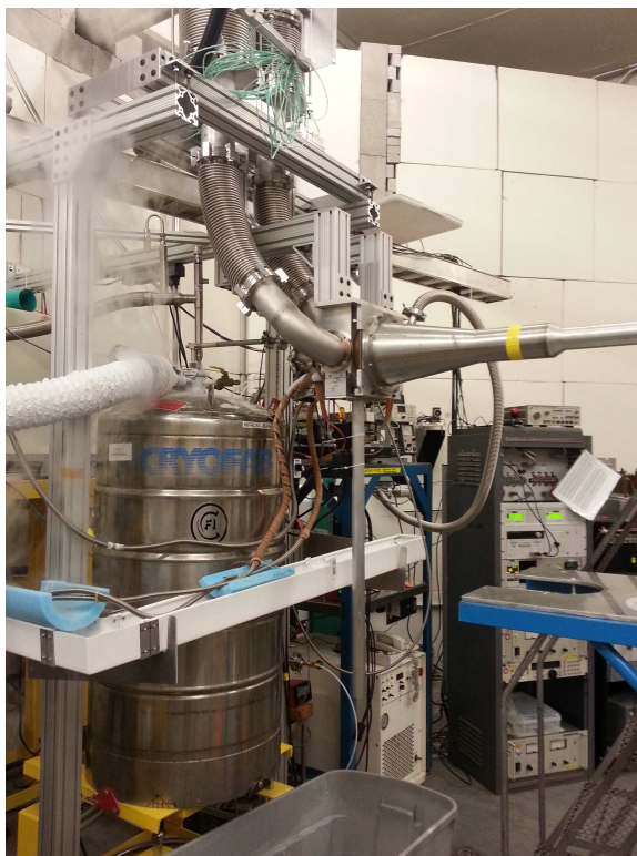
Figure 2.10: Picture of the HIFROST target's cooling system in its first cool down test in September 2013
