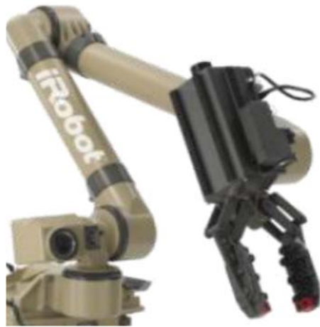
Figure 4.7 Manipulator arm of rescue robot (Multi mission modular robot, 2014)
