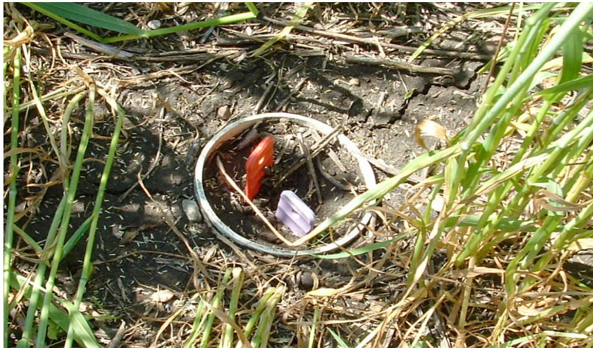
Figure 1. PRS probes placed in PVC cylinder in field in wheat crop.
