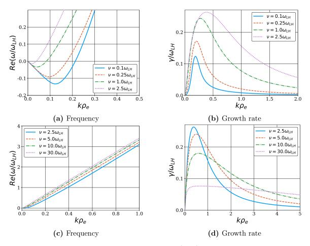
**Figure 4.2:** Solution to the dispersion equations (4.14) for different values of electron collision frequency  $\nu$  and typical Hall truster parameters:  $v_{i0} = 4.45\omega_{LH}\rho_e$ ,  $v_{e0} = -1.33\omega_{LH}\rho_e$ .
