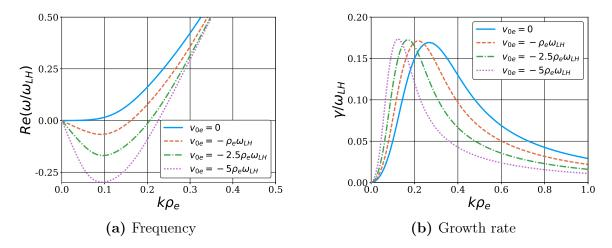
**Figure 4.4:** Solution to the dispersion equations (4.14) for different values of equilibrium electron velocity and typical Hall thruster parameters  $v_{i0} = 4.45\omega_{LH}\rho_e$ ,  $\nu = 0.25\omega_{LH}$ .
