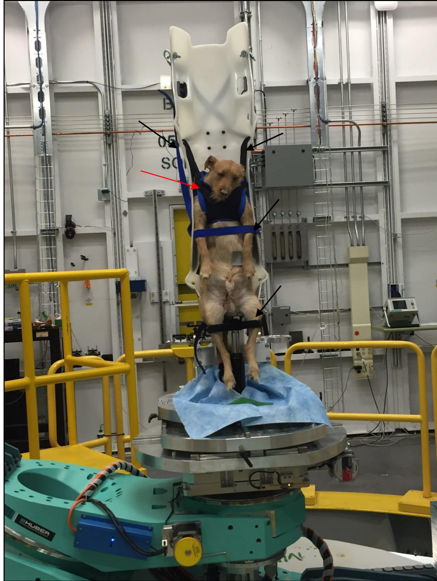
Figure 5.4: An example of a dog cadaver secured into the canine positioning device by the Walkabout™ front harness. The harness is indicated by a red arrow, and the hook-and-loop straps indicated black arrows.
