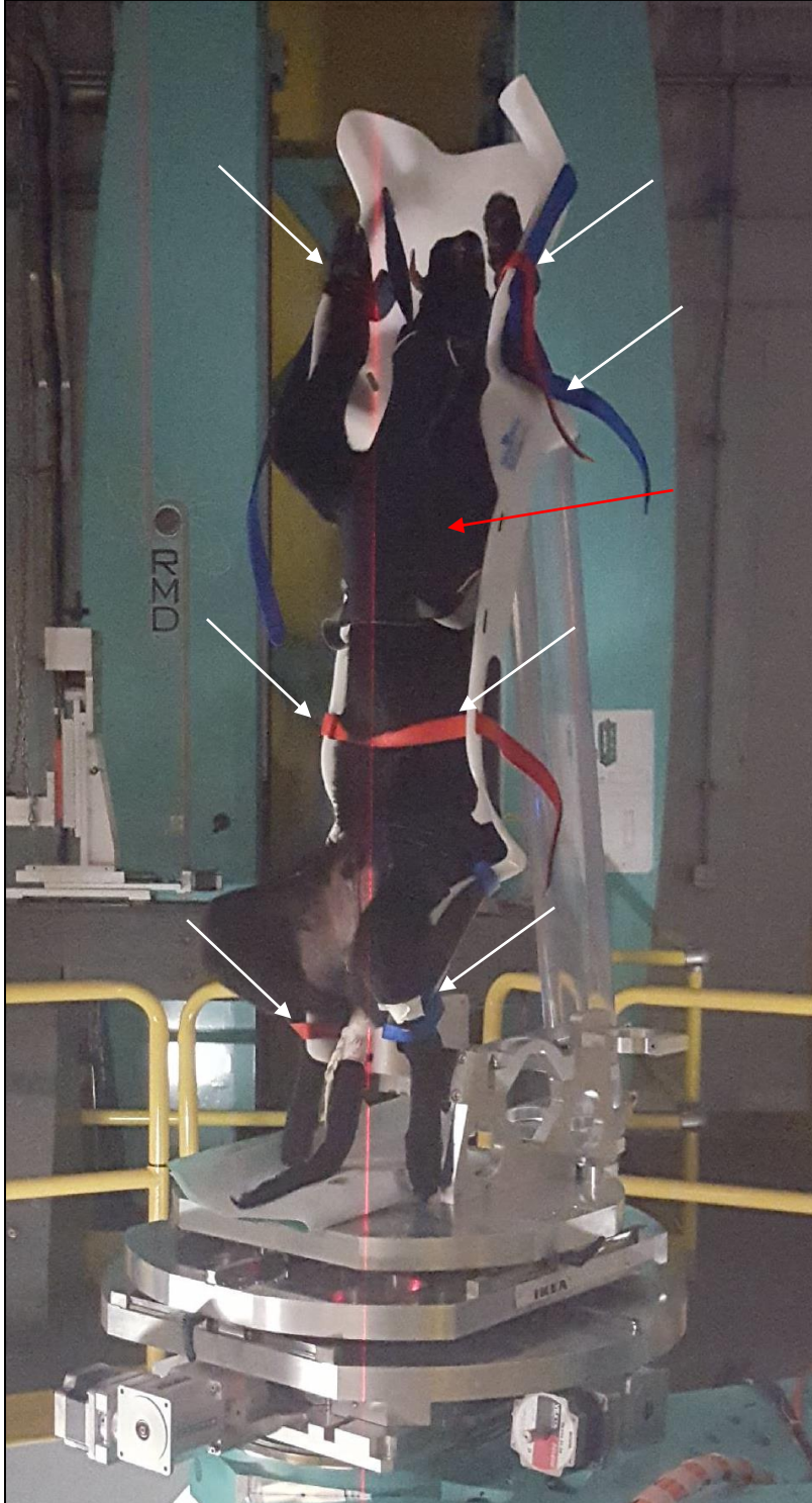
Figure 5.3: Cadaver two secured using the Ruffwear® Load Up™ harness (red arrow), and the hook-and-loop straps (white arrows) within the positioning device for imaging.
