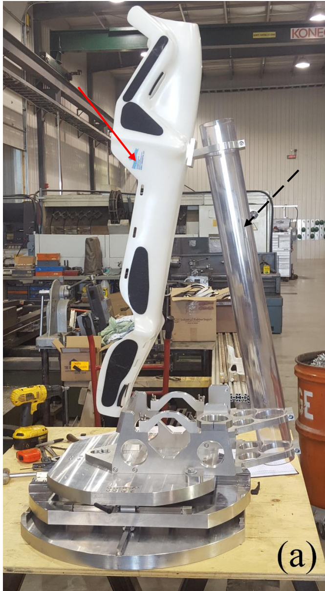
Figure 4.14: (a) A side view of the final design of the canine positioning device, with the Pawitioner indicated with a red arrow. The polycarbonate support tube is indicated with a dashed black arrow. (b) A side view of the final draft design approved by the USPT, with the arrows indicating the same structures as in (a).
