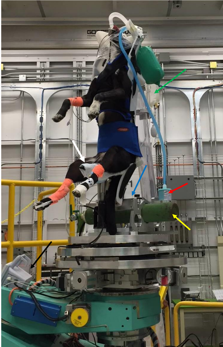
Figure 5.13: An image of a live dog set up for imaging at the CLS BMIT. The oxygen tank, vaporizer, IV drip and gas filter are indicated with a yellow, blue, green, and red arrow, respectively. The monitoring equipment is indicated with a black arrow. The modified seat can also be seen in this image, indicated with a white arrow.
