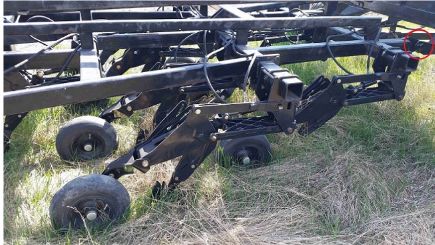
Figure 2.5: The front two ranks of row units are pictured. The pivot between the front boom and subframe is circled in red. This allows the subframe with row units to pivot separately from the front boom.
