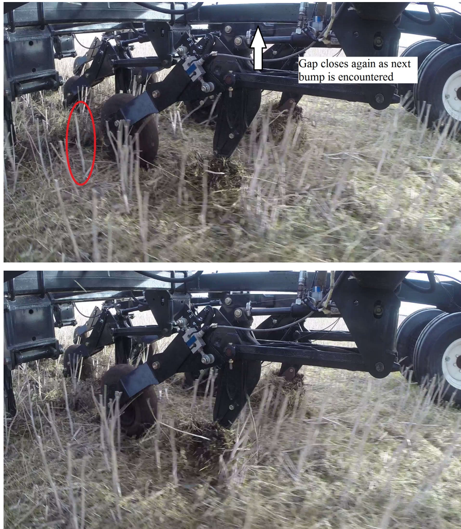
Figure 4.18: As the packer wheel reached the point where the row unit was previously at its maximum height while passing over the residue clump, the row unit began to move upward. In the bottom image, the packer wheel has passed the marker stalk and has moved downward again.
