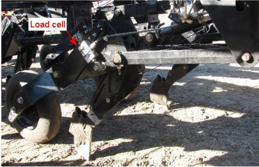
Figure 4.2: The load cell used to measure a component of the resultant packer wheel force is visible on the row unit body.
