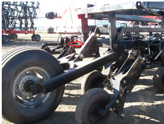
Figure 2.7: The tail wheel supported the rear end of the subframe to which all row units mount. It connected to the subframe via a 4-bar linkage system.
