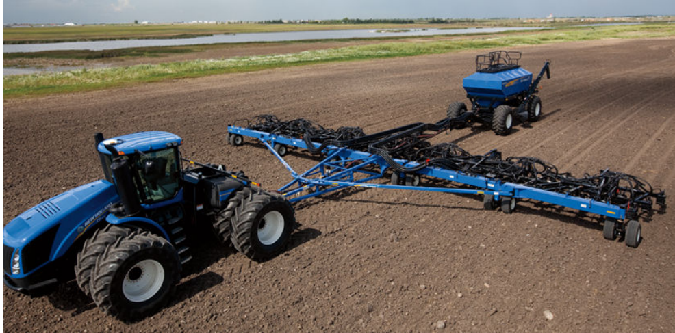
Figure 1.1: A New Holland P2070 Precision Hoe Drill unfolded into the working configuration, with the bulk product air cart towed behind. Image credit: www.newholland.com .
