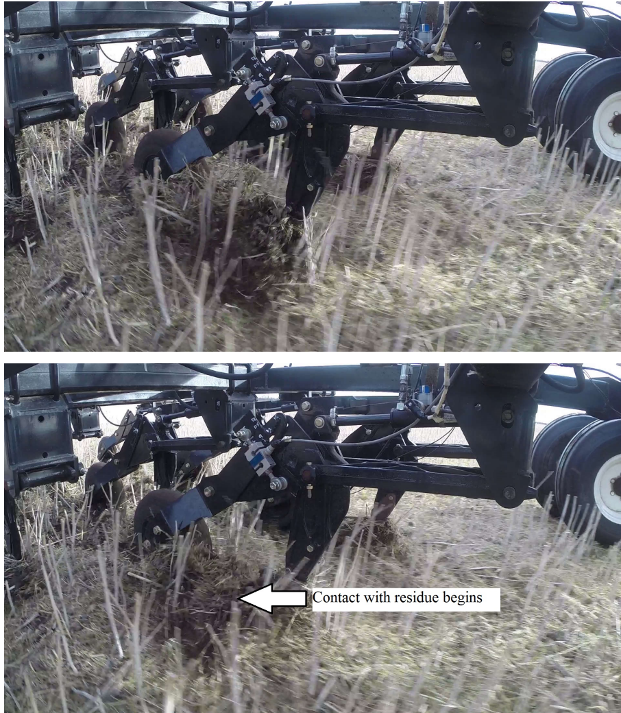
Figure 4.16: The clump was pulled from the opener in the top image. The row unit began to move upward in the bottom image as the packer wheel engaged the residue.
