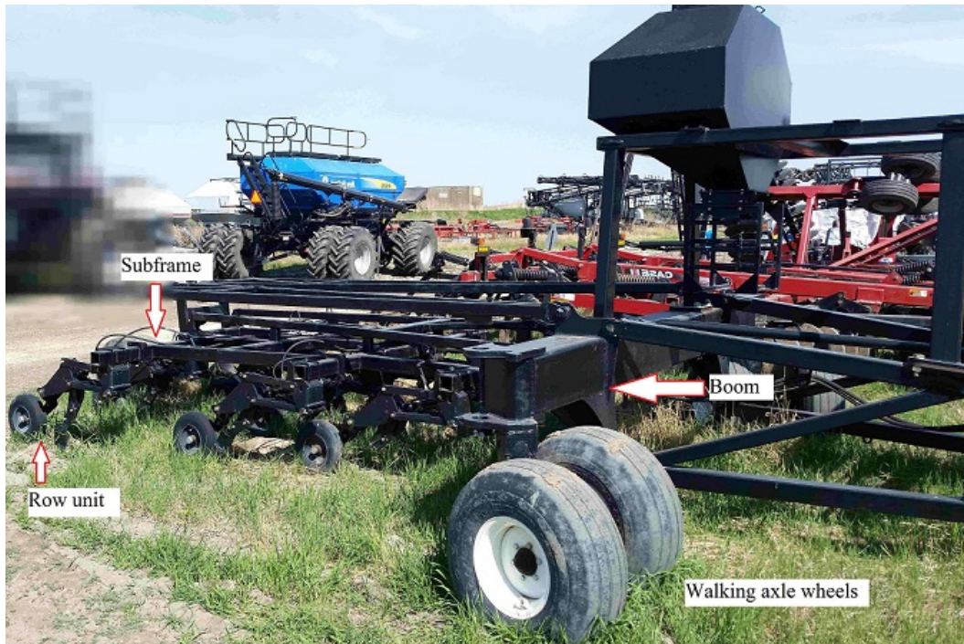
Figure 2.2: A side view of the plot drill. 3 ranks of row units are mounted to a subframe of the plot drill. 12 row units are mounted on the plot drill.
