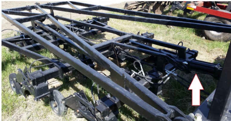
Figure 2.8: The frame hydraulic cylinder extended between the front boom and the subframe. The pressure applied to this hydraulic cylinder changed the vertical load carried by the tail wheel, walking axle wheels, and tractor hitch. The large frame structure above the subframe was part of the production-model hitch system used to pull an air cart.
