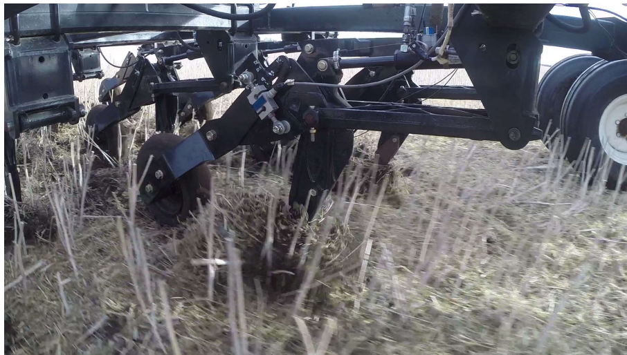
Figure 4.15: Residue continued to collect and extend up the front of the opener. The clump became wider in the top image. The residue clump began to release and pass alongside the opener in the bottom image.
