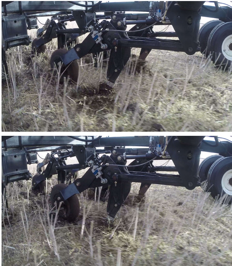
Figure 4.14: The hoe opener before crop residue started accumulating residue is shown in the top image. The opener begins to push residue along the soil surface in the bottom image as an area of heavier residue was encountered.
