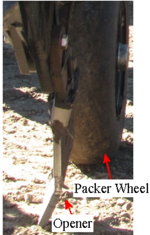
Figure 2.4: The profile of the opener is evident, with the packer wheel in the background. Note the slight bend in the opener creating a “winged” portion below the soil surface.
