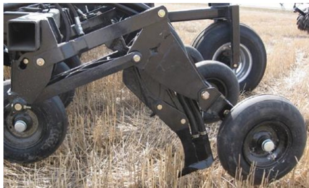
Figure 2.2: A typical air seeder row unit. Image credit: www.caseih.com . (Accessed February 2018)
