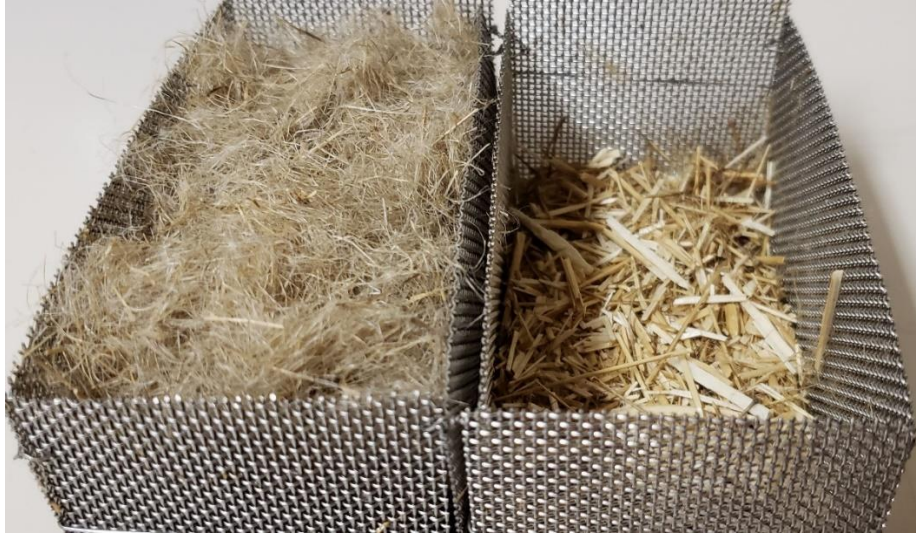
Figure 4.17. Four grams of flax fibers (left) and four grams of flax shives (right).
