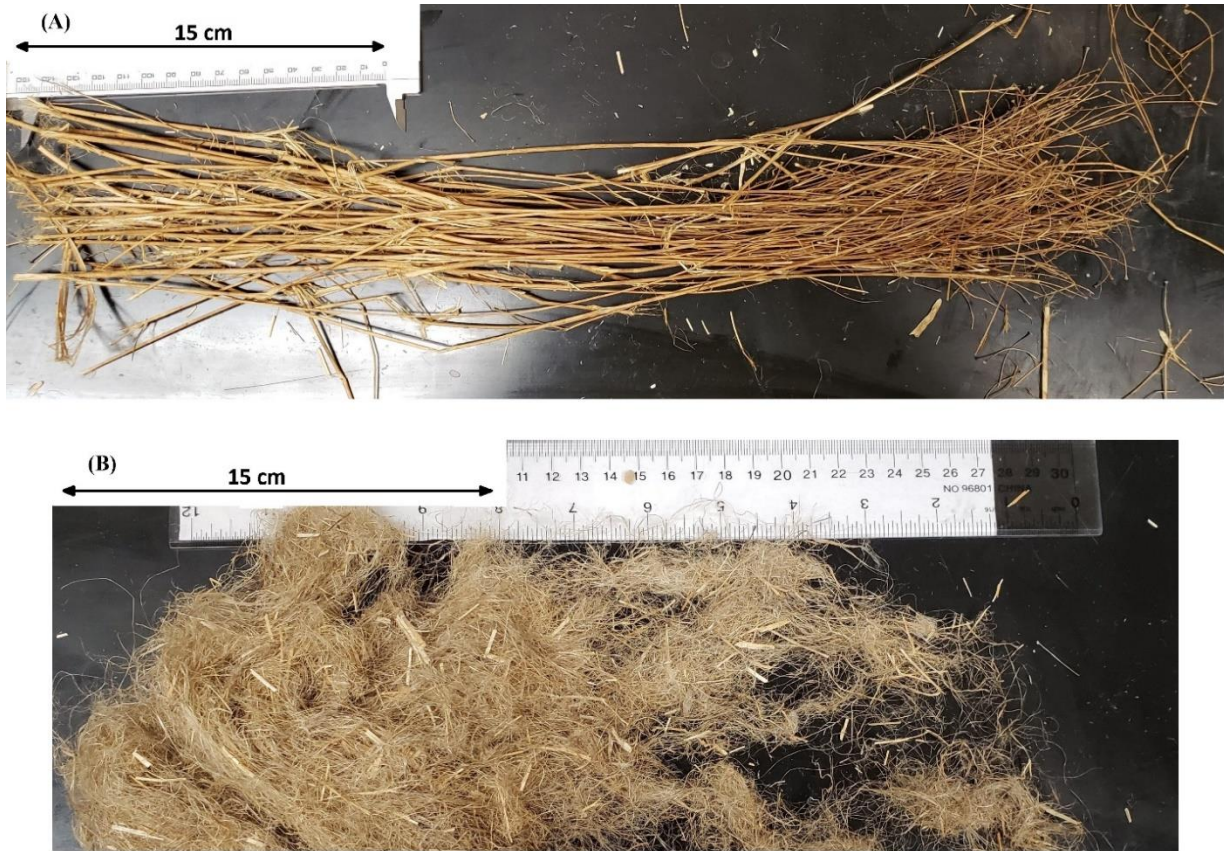
Figure 3.1. Sample batch of as-received flax straw (a) and processed flax fiber (b).
