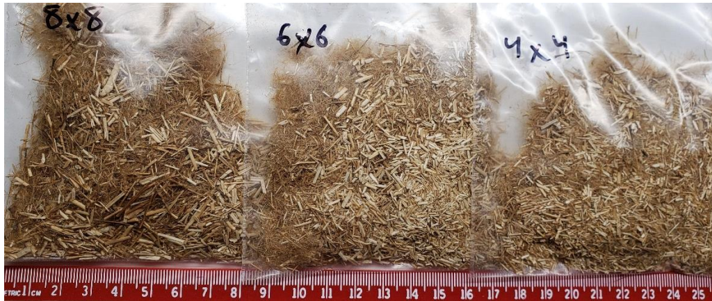
Figure 4.8. The 4-gram samples made with the knife milling machine using three sieve sizes.
