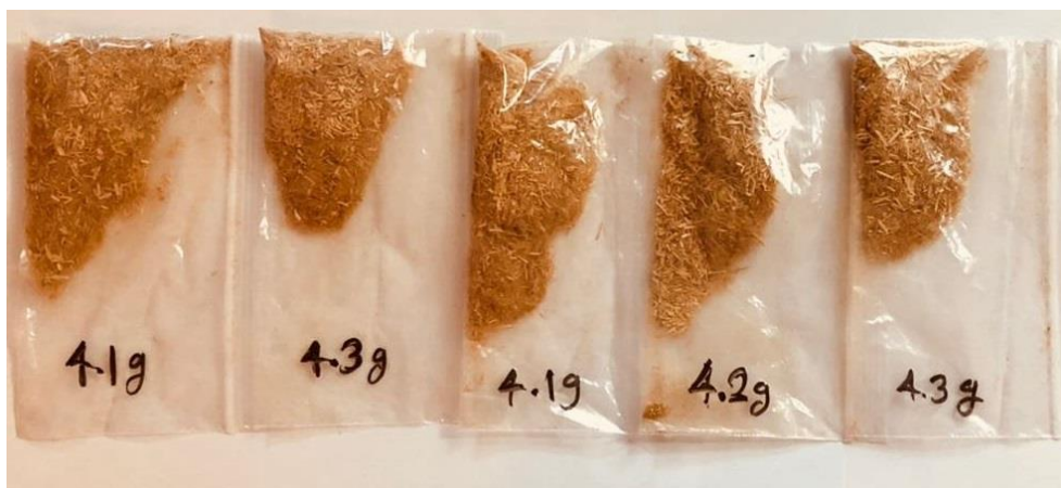
Figure 3.6. Individual packages for each cut sample containing the sample fiber to shive ratio.
