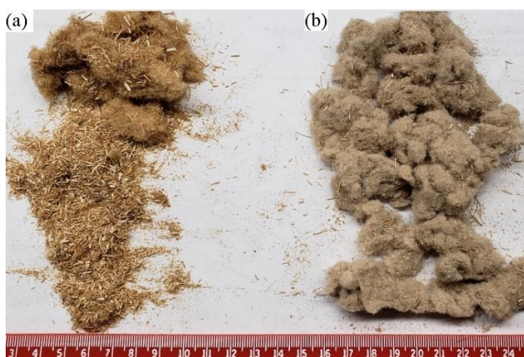
Figure 4.7 Ground and sieved batch of flax straw (a) and flax fiber (b).
