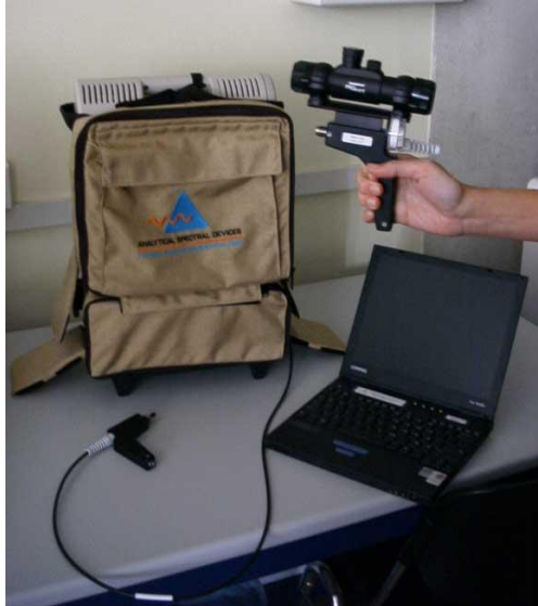
Figure 2. 8. Picture of portable spectroradiometer (model ASD FieldSpect Pro ) showing the main spectroradiometer unit, fore-optic lead device, and laptop used in device operation.
