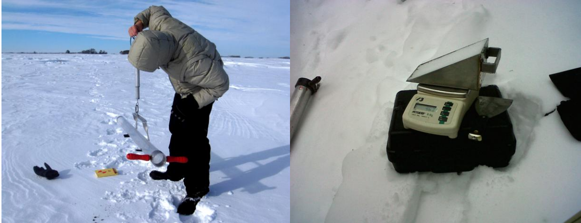
Figure 2. 10. Methods used for measuring snow density in the field: ESC-snow tube weighted by calibrated spring scale (left), and volumetric snow cutter from sample taken from dug snow pit weighted by electronic balance (right) (left photo courtesy of X. Fang).
