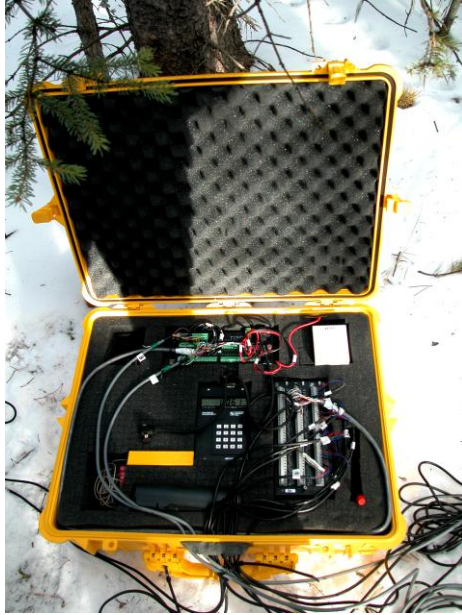
Figure 2. 6. Portable data logger system used in the control of array radiometer sensors and data recording.
