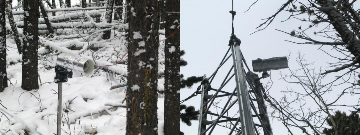
Figure 2. 9. Installations of infrared thermocouples measuring trunk surface temperature (left) and crown foliage temperatures (right).
