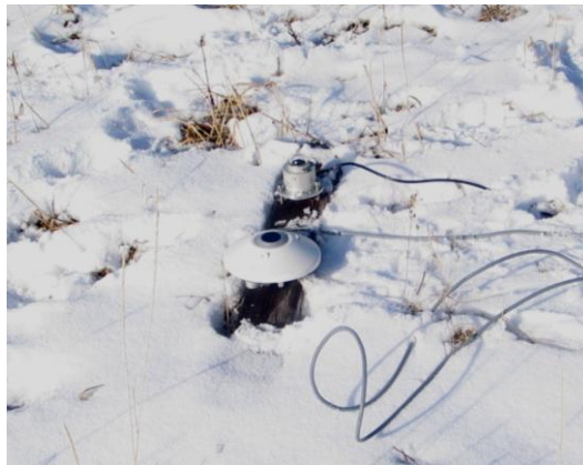
Figure 2. 7. Paired pyranometer-pyrgeometer sensors at nearby clearing for observations of reference shortwave and longwave irradiance.
