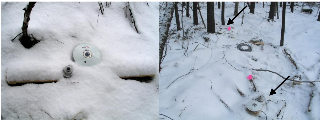
Figure 2. 5. Paired pyranometer and pyrgeometer radiometers shown inclined with the ground slope at the Southeast-facing Pine Forest site (SPF) (left), and at the Level Pine Forest site (LPF) (right).
