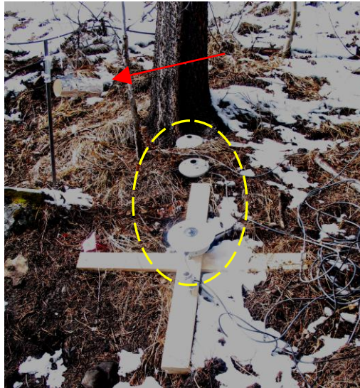
Figure B1. Picture showing the instrumentation set-up used in the empirical optimization of the b_d biomass depth used to approximate the thermal capacity of the outer biomass layer of the forest stand (infrared thermocouple measuring trunk surface temperature indicated by arrow, with pyranometers and pyrgeometers indicated by yellow dashed line).
