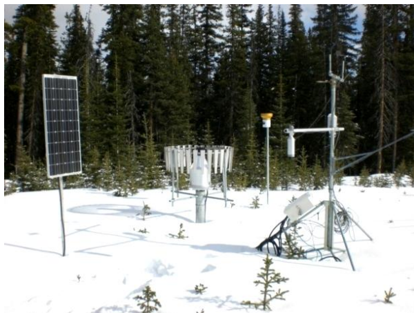
Level Spruce Clearing site (LSC) showing tower for observations reference radiation (left) and near-surface meteorological observation installation (right).
