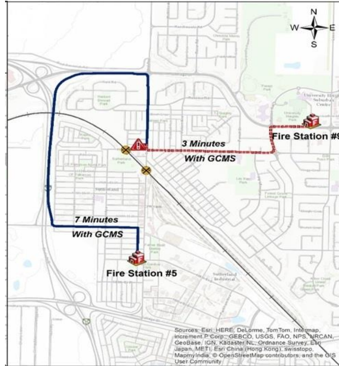
Figure C-3. Fire Engine Dispatch Routes to an Incident with/without Grade Crossing Blockage and with GCMS
