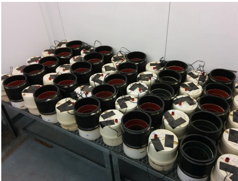
Fig. 4.1: Incubation chamber setup in the phytotron between sampling times. During each day of sampling lids are sealed onto the top of each chamber containing soil and the gas samples are taken 1, 3, and 5 hrs after sealing.
