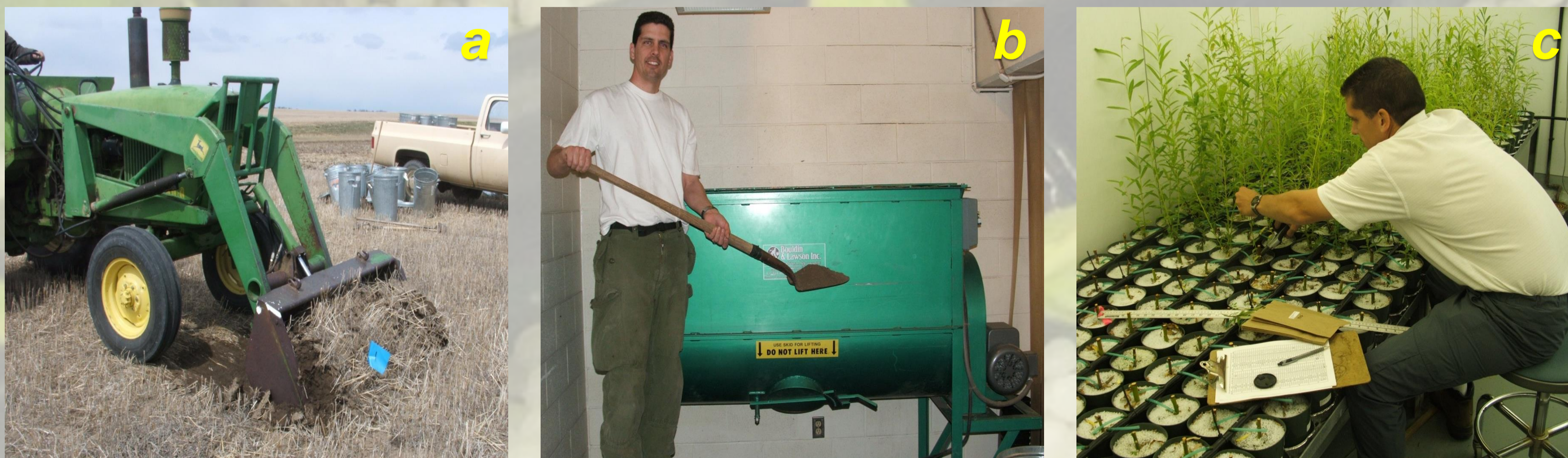
Figure 1. Collecting soil along a saline hillslope catena near Central Butte, SK (a), blending air-dried soils to achieve desired salinity levels (0.8, 3.6, 5.0, and 8.0 dS/m) (b), and assessing willow growth after 60 days (c).
