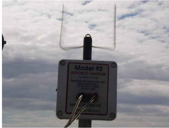
Figure 3.7 Rotorod collector mounted on the electric motor
