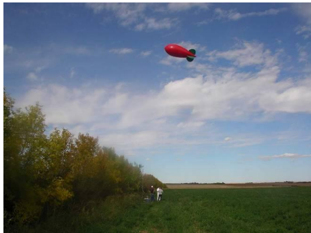
Figure 3.6 Polyethylene line suspended by the helium blimp
