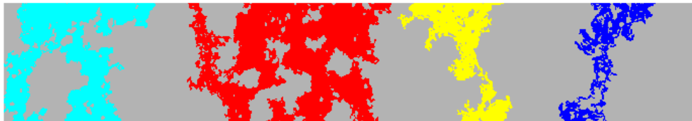
Figure 4.3 Processed image from the binary image in Fig. 4.2 that shows the isolated connected preferential flow paths in different colours.
