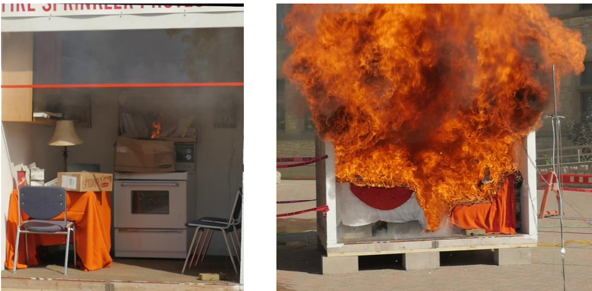
Figure 1.11 Images near peak temperature measurements for fire demonstrations in (left) kitchen and (right) bedroom constructions (Fulton, et al. 2017a)
