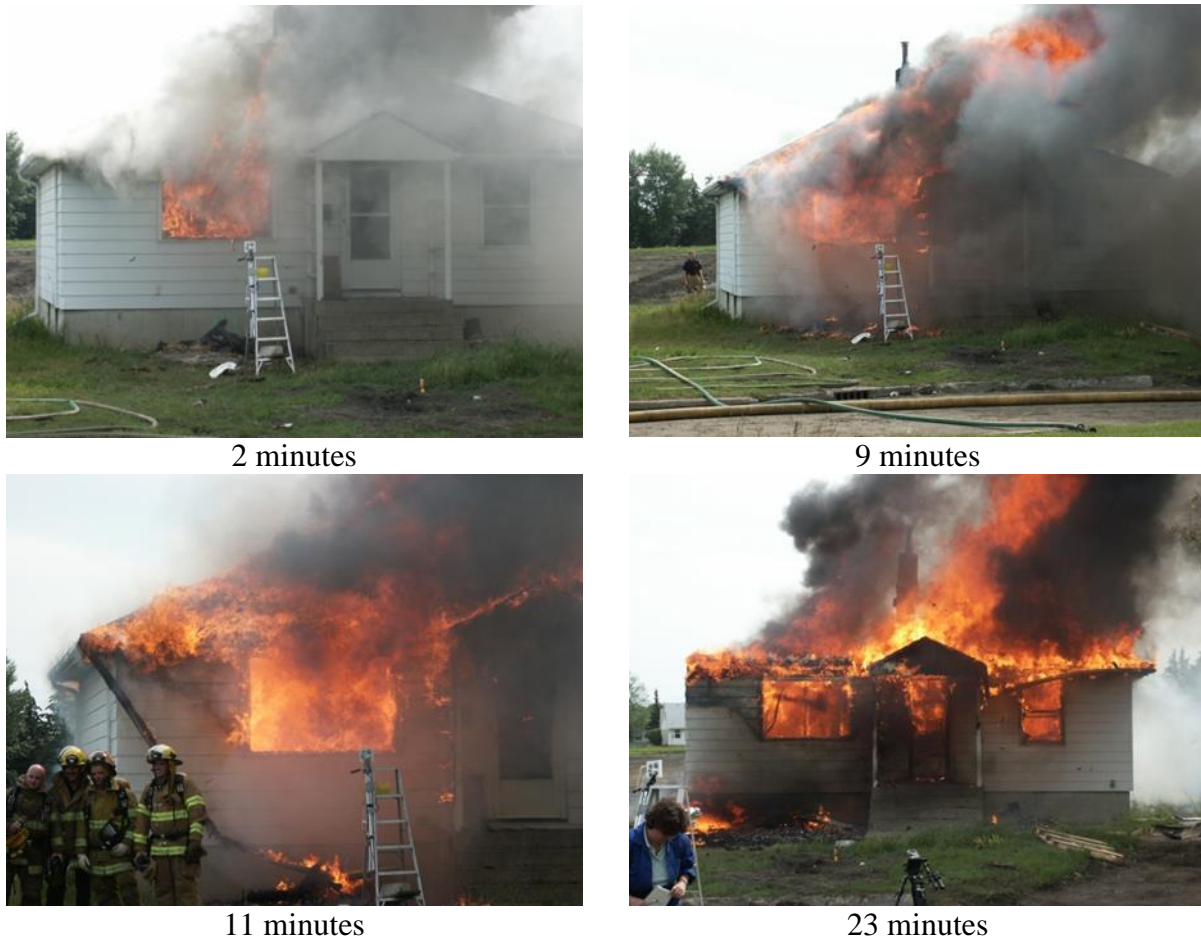
Figure 1.5 Fire development from the Edmonton full scale house fire (Threlfall, et al. 2004)
