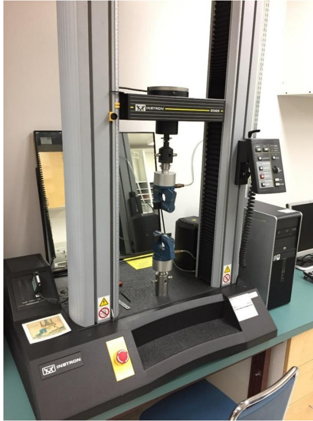
Figure 2.8 Instron 5565 tensile testing apparatus located in an environmentally controlled laboratory in the Department of Human Ecology at the University of Alberta
