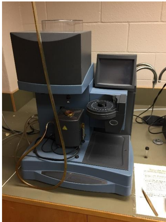
Figure 2.4 Q5000 TGA testing apparatus
