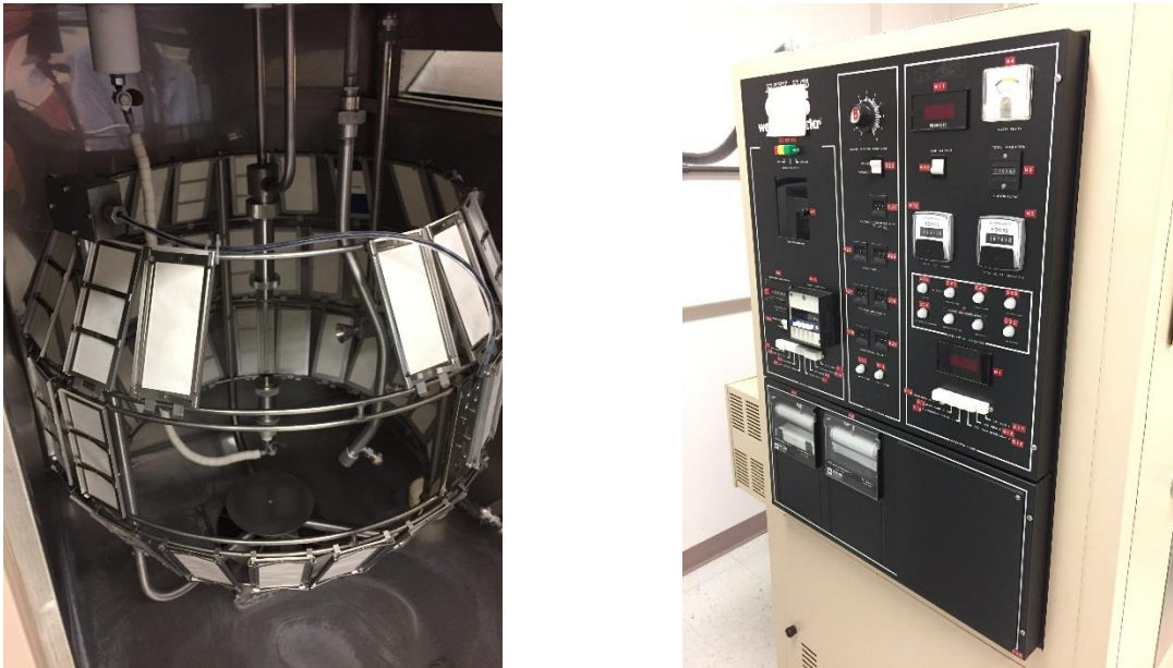
Figure 2.7 Interior view of the Weatherometer UV chamber (left) and side-mounted control panel (right) at the University of Alberta
