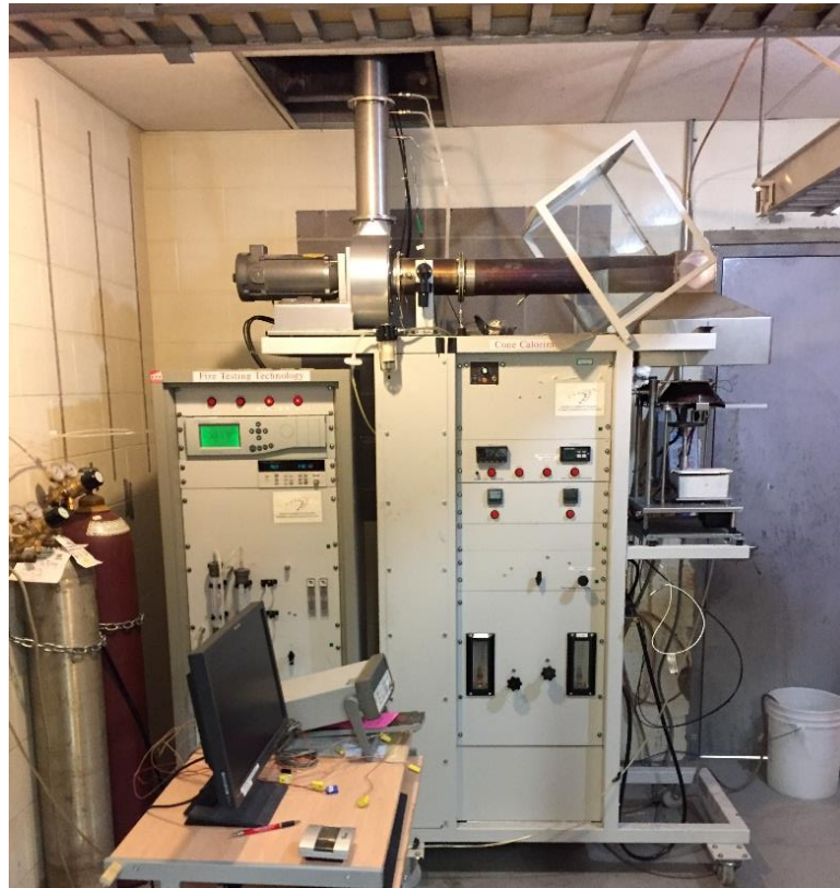
Figure 2.5 UofS cone calorimeter in horizontal orientation
