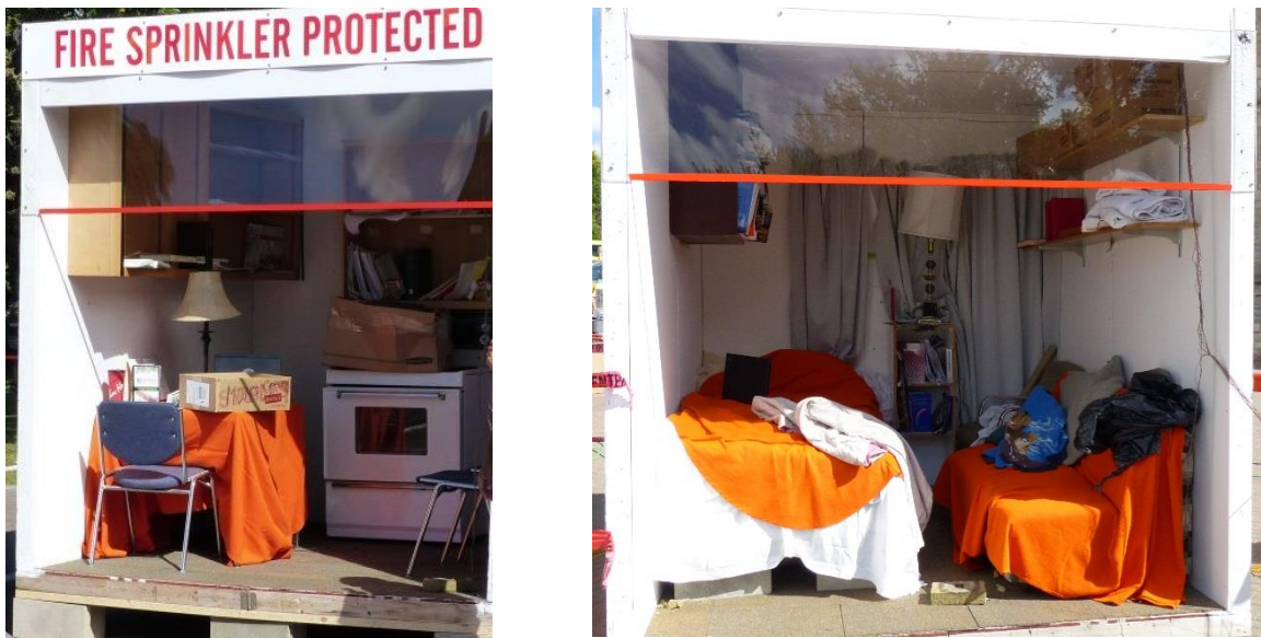
Figure 1.10 Pre-test images of the constructed (left) sprinklered kitchen and (right) unsprinklered bedroom (Fulton, et al. 2017a)
