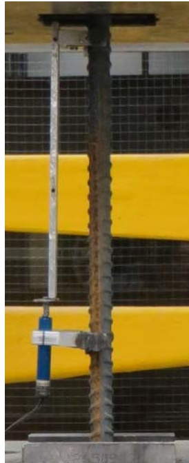
Figure 3.30: Extensometer Used to Measure Displacement of the Bar Sample of an 200 mm Gauge Length.
