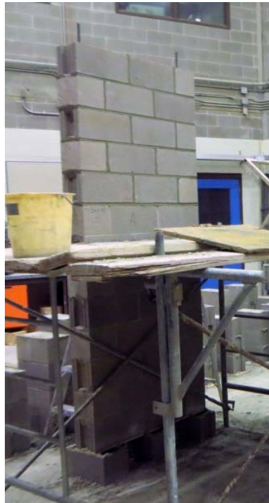
Figure 3.21: Newly Completed Wall Splice Specimen.
