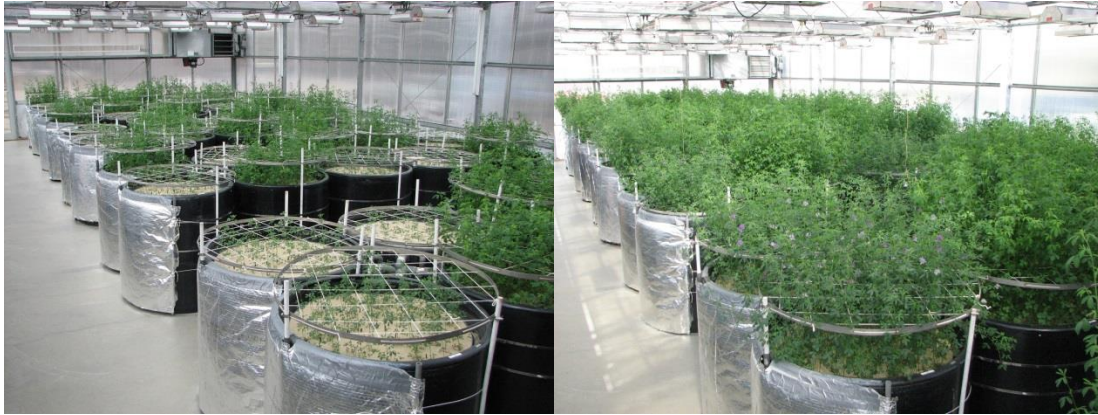
Figure 7. Salinity Lab, grow tanks which are capable of growing crops to maturity. The dimensions of each tank are 1.0 m high by 0.95 m in diameter with a growing surface area of 0.57 m 2 .
