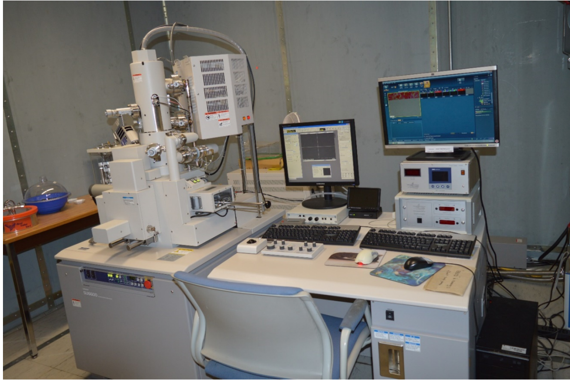
Figure 3.7. Hitachi SU6600 SEM equipped with an Oxford X-Max Silicon Drift EDS and Oxford NordlysNano EBSD.
