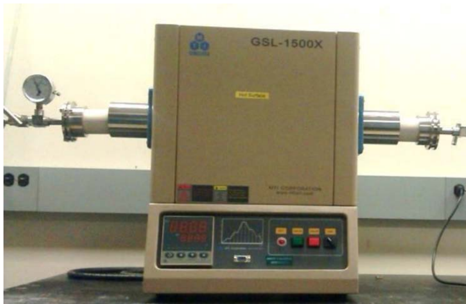
Figure 3.3. Tube furnace used for oxidation in air.
