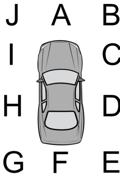
Figure 5-2. Possible impact locations on the subject vehicle. Location of obstacle, Motorist 2 , is coded A – J in relation to the subject vehicle. Impact locations B, C, D, & E were coded as right and locations G, H, I, & J were coded as left.
