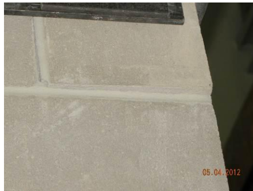
Figure 4.37: Photograph of the debonded half-block in the top course of Specimen RD2
