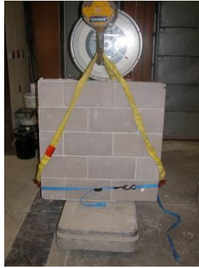
Figure 4.53: Weighing of wall section extracted from Specimen IS4
