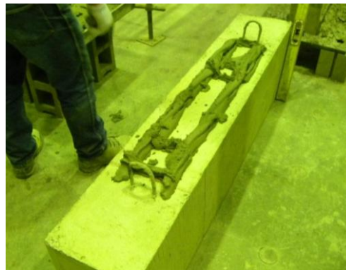
Figure 3.8: Concrete base with initial mortar bed joint
