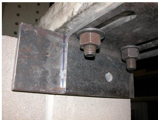
Figure 3.17: Realistic pin showing the top connection
