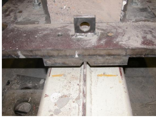
Figure 3.16: Ideal pin showing the bottom knife-edge connection.
