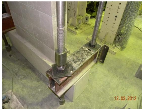
Figure 3.15: Realistic pin support specimen showing the bottom connection
