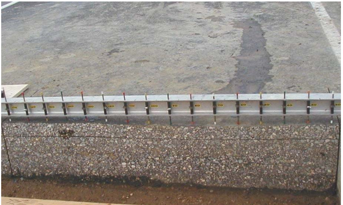
Figure 2.8 Cross Section of Asphalt Concrete Layer Isolated Wheel Path Rutting Due to Viscoplasticity (Courtesy of DHT)
