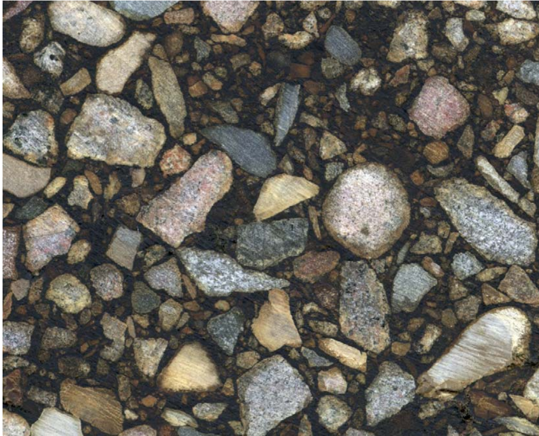
Figure 2.9 Coarse Dense Graded Hot Mix Asphalt Concrete Mix Particulate Composite Cross Section
