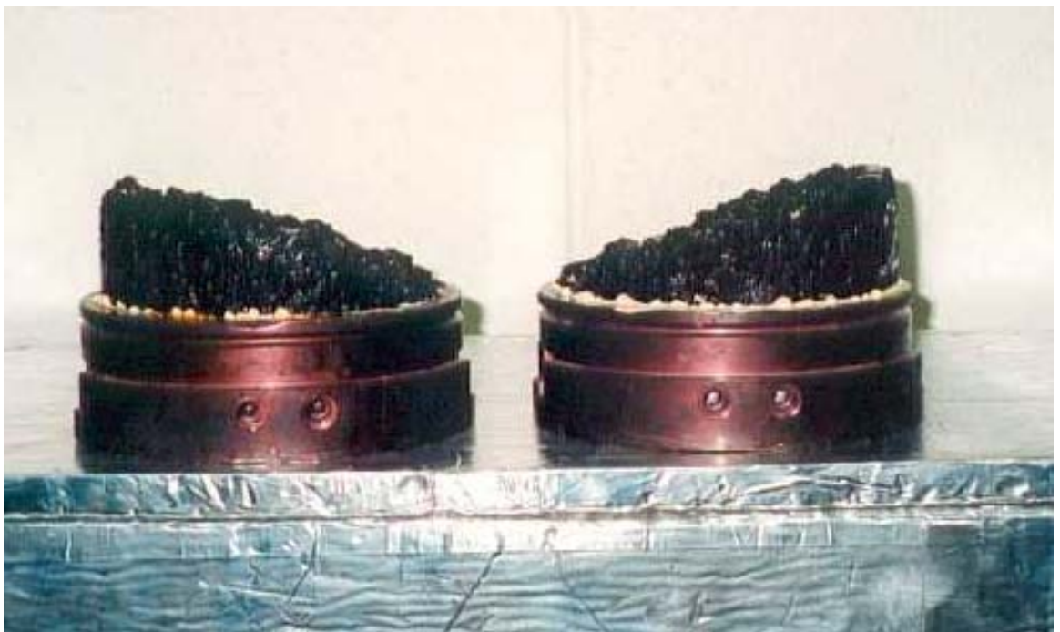
Figure 2.46 Superpave Repeated Shear Tester Failed Sample
