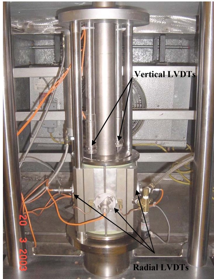
Figure 2.50 Rapid Triaxial Test Cell Lowered Over Asphalt Concrete Sample
