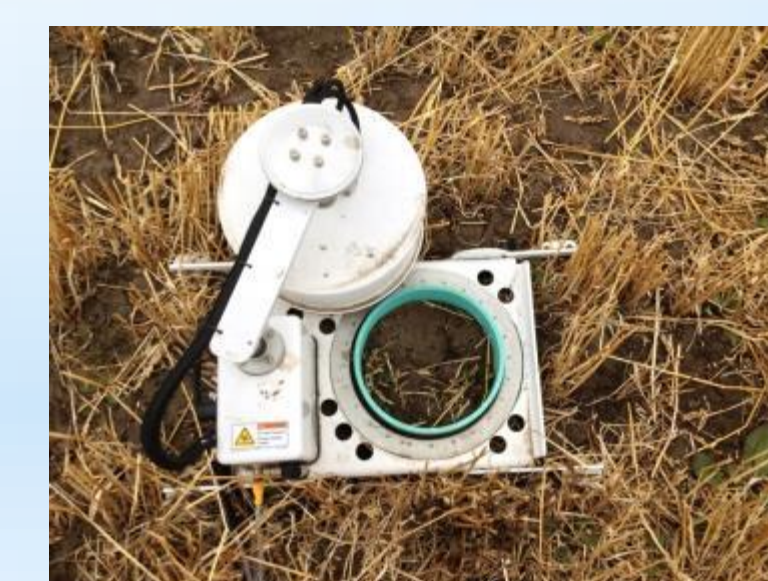
Fig 5. Greenhouse gas (N 2 O, CO 2 & CH 4 ) emissions measured with the Gasetm DX-4015 FTIR-multigas analyzer connected to a Li-Cor 8100-104 long-term flux chamber via a LI-8150-16 multiplexer.
