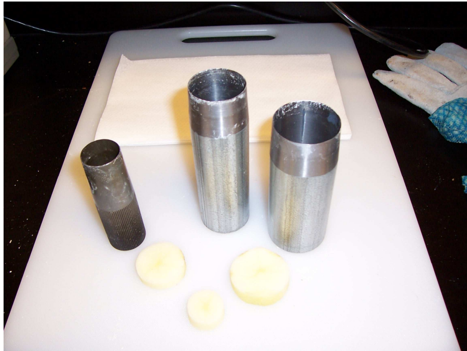
Figure 3.3: Sweetpotato sample sizes and cylindrical borers used to cut samples.
