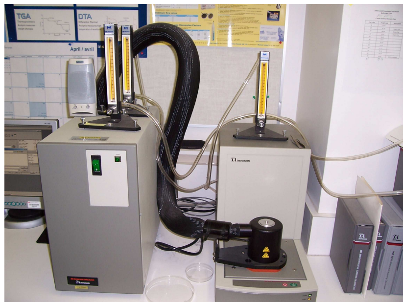
Figure 3.2: DSC 2010 used for specific heat measurement of sweetpotato.
