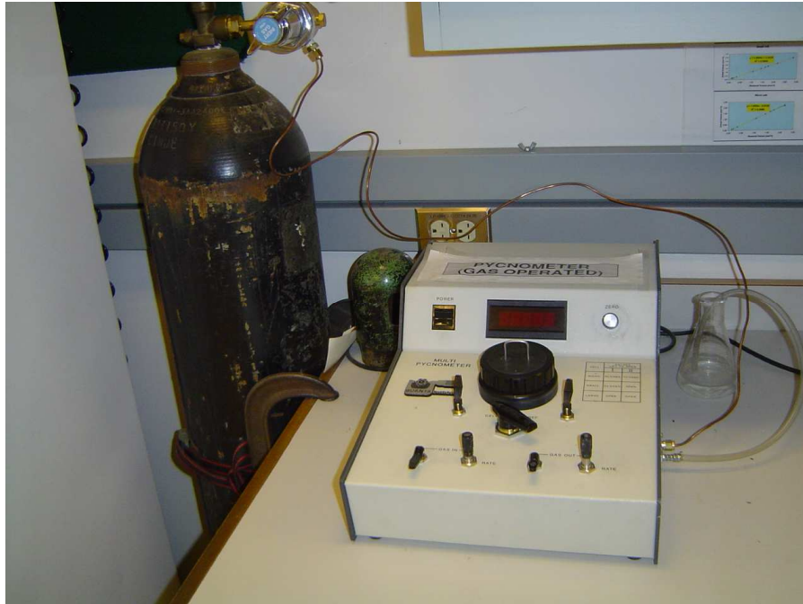
Figure 3.1: Multipycnometer used to measure density of sweetpotato.
