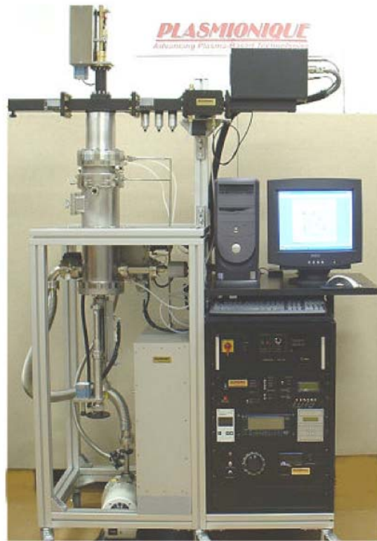
Figure 3-3. MPCVD reactor (MWPECVD 1250UOS, 2.45 GHz).
