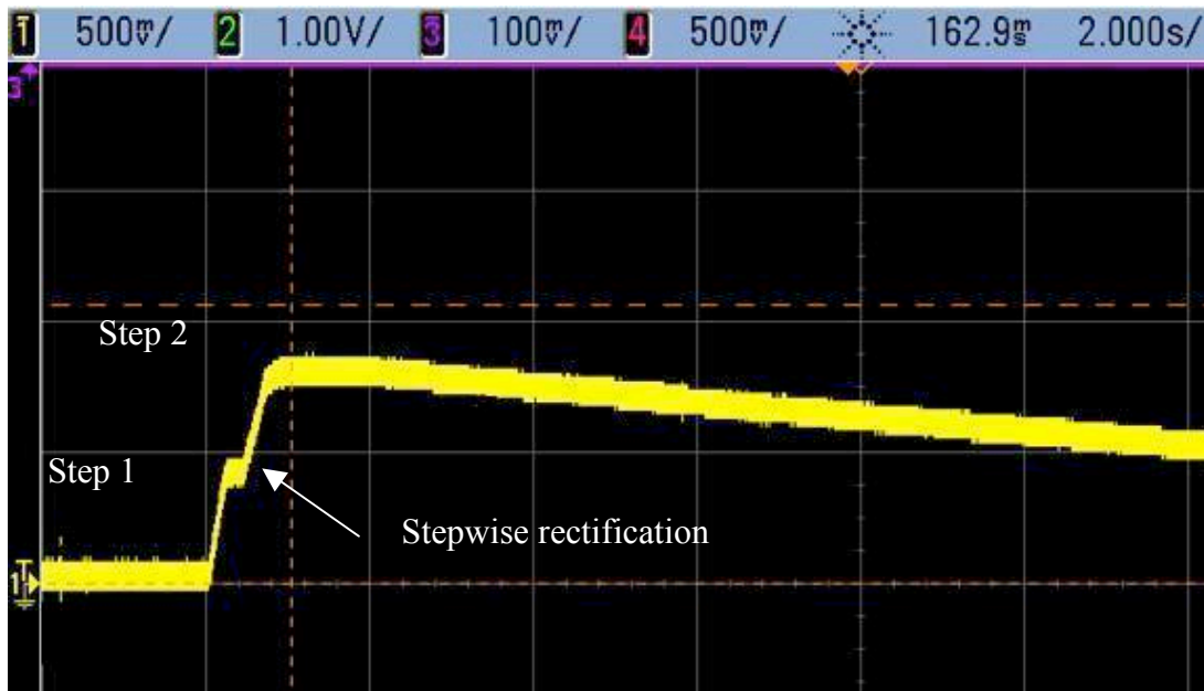
Figure 7.4.2.2: Close-up of voltage across 2.2 \mu F capacitor demonstrating rectification of double polarity voltage produced by the PVDF film when subjected to a mallet strike
