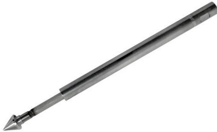
Figure 7. AMS® Gas Vapor Implants used for sampling groundwater.
