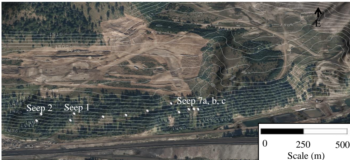
Figure 16. Groundwater springs (white dots) along the southern extent of the catchment with labels denoting springs that flowed continuously throughout the year. Contour lines represent 2-m intervals in surface elevation (masl).
