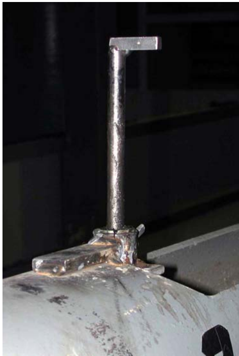
Figure F.20: Depth of flow measurement gauge on the 156.7 mm flume test section
