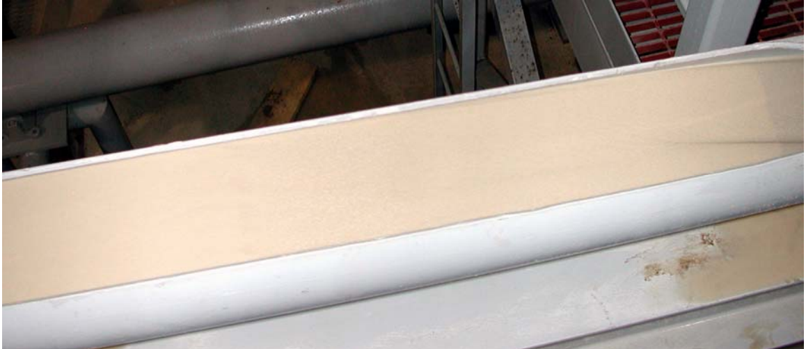
Figure F.3: Deposit in the 156.7 mm flume test section with the 25% v/v sand-water tests
