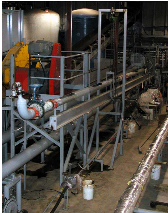
Figure F.6: View of the 156.7 mm flume circuit from inlet to outlet (left to right)
