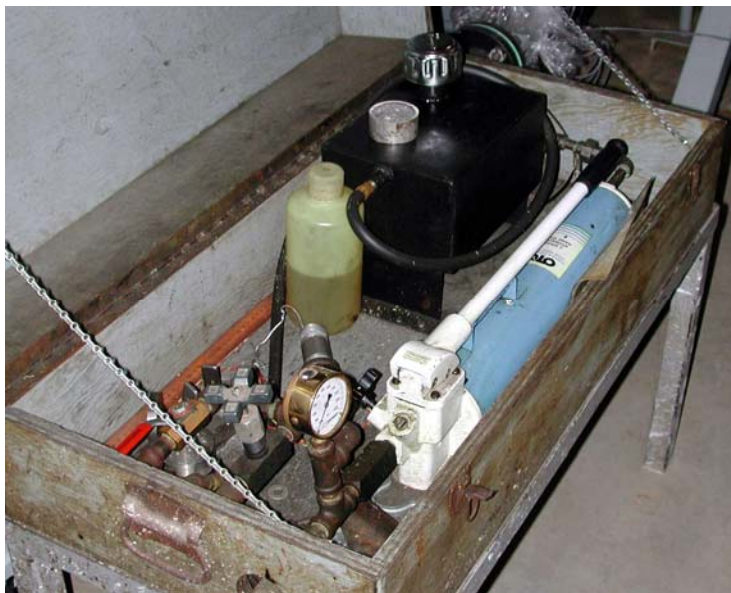
Figure F.24: Hand pump apparatus used to traverse the Ronan gamma ray densitometer on the 156.7 mm flume
