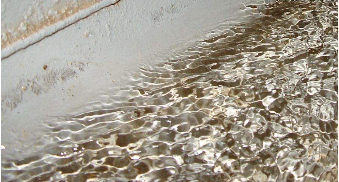
Figure F.1: Rippled free surface of a turbulent water flow in the 156.7 mm flume test section
