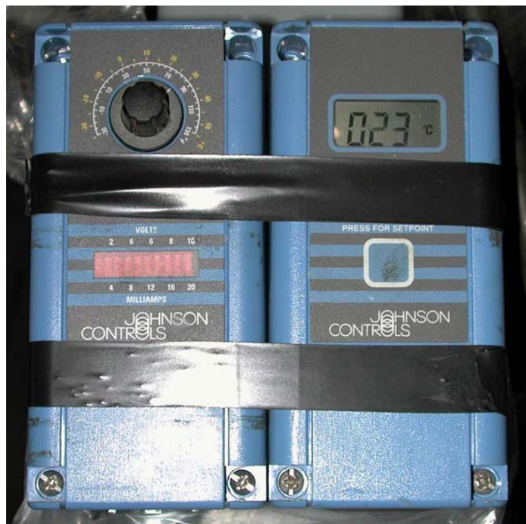
Figure F.16: Proportional controller for the system temperature on the 53 mm feed pipe used in the 156.7 mm flume experiments
