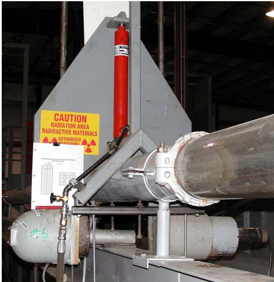
Figure F.23: Ronan traversing gamma ray densitometer on the 156.7 mm flume
