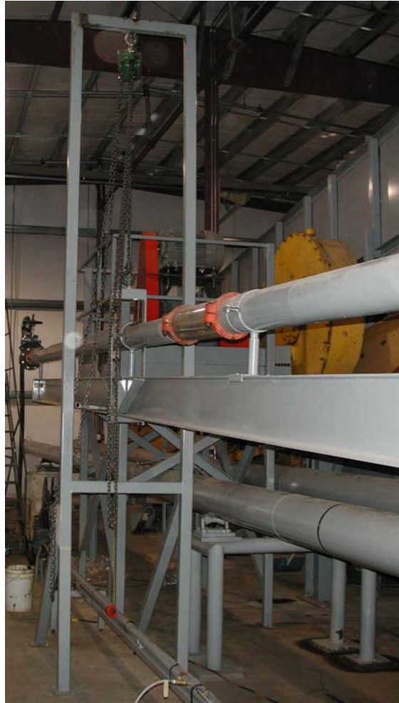
Figure F.7: View of the 156.7 mm flume circuit winch and hoisting apparatus
