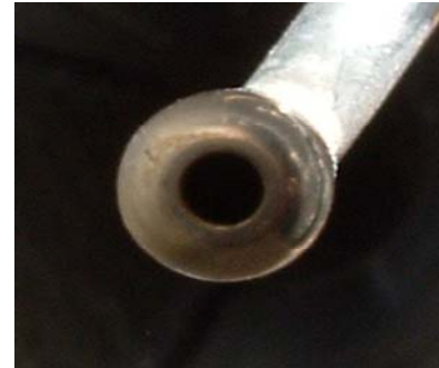
Figure C.2: Sample digital photograph of the flume Pitot-static tube tip (2006)
