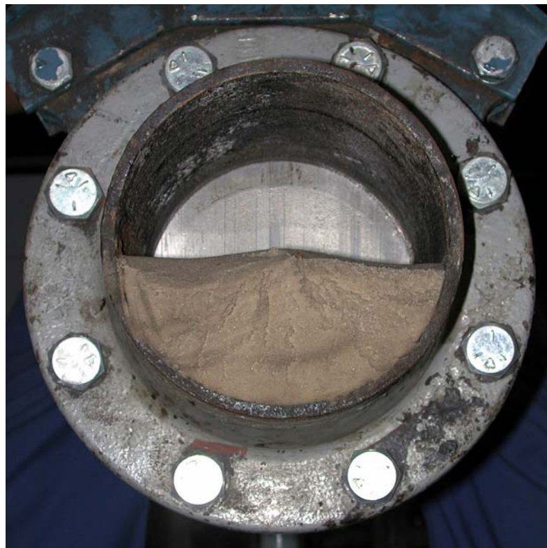
Figure F.2: Deposit in the old 156.7 mm flume inlet with the 25% v/v sand-water tests
