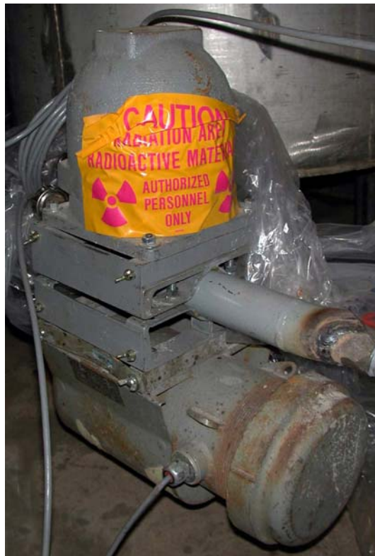
Figure F.12: Ronan densitometer on the 53 mm feed pipe used in the 156.7 mm flume experiments
