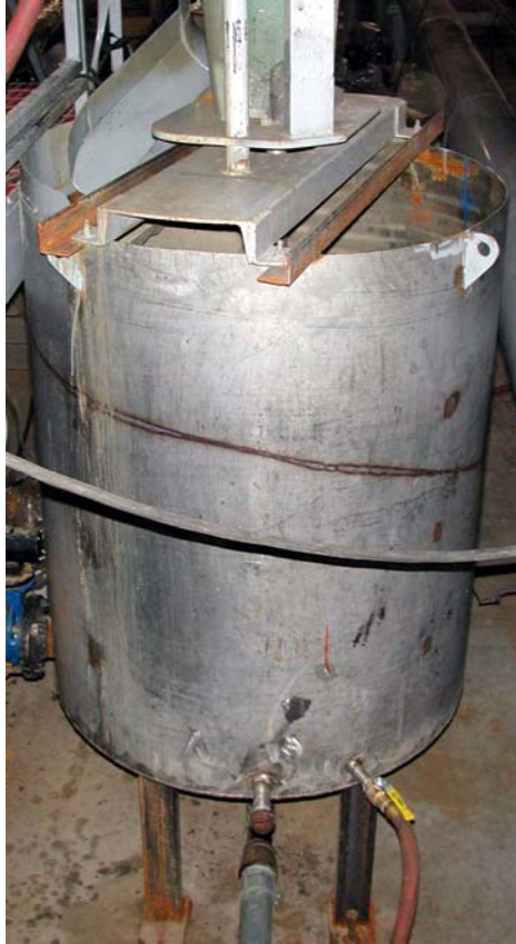
Figure F.25: Stand tank for the 156.7 mm flume circuit
