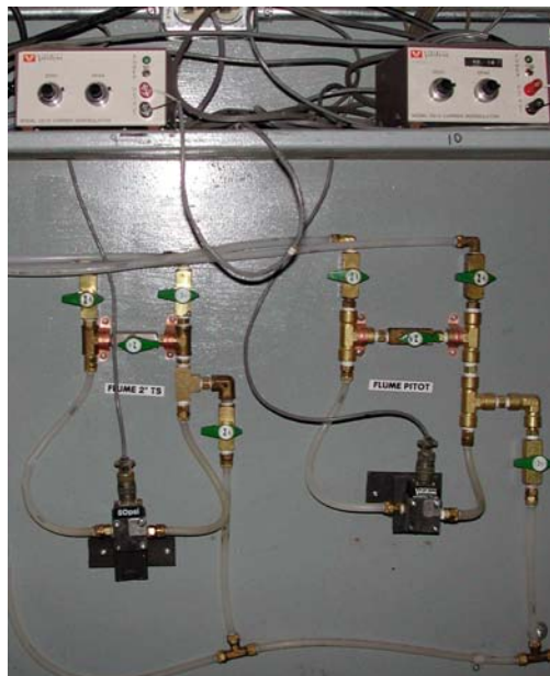
Figure F.14: Validyne pressure transducer bodies and demodulators used in the 156.7 mm flume experiments
