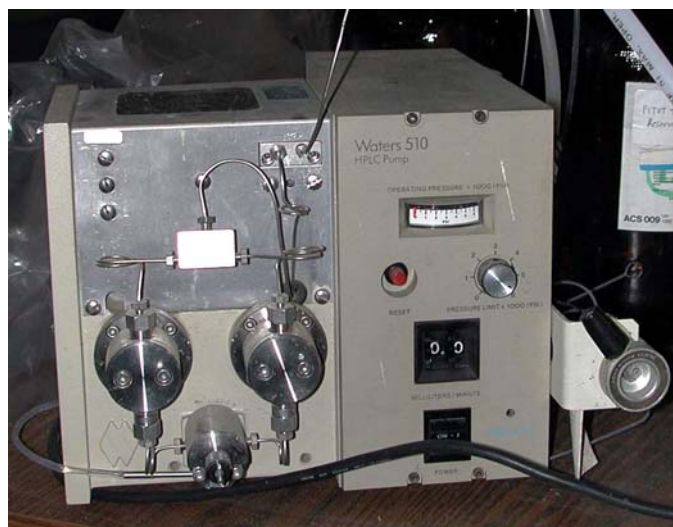
Figure F.22: HPLC purge pump for the Pitot-static tube measurements during the 156.7 mm flume experiments
