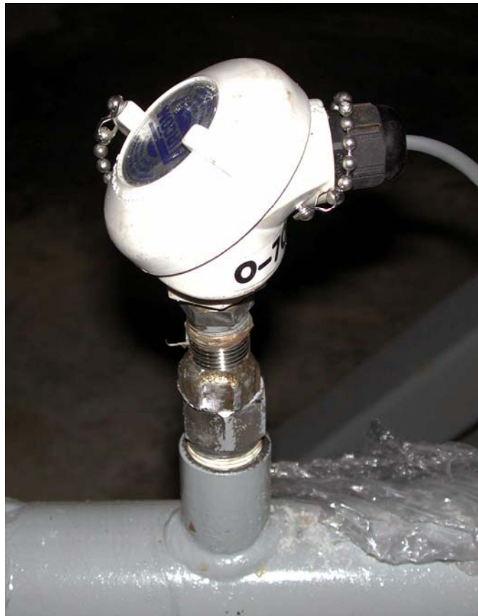
Figure F.13: Aircom temperature sensor on the 53 mm feed pipe used in the 156.7 mm flume experiments
