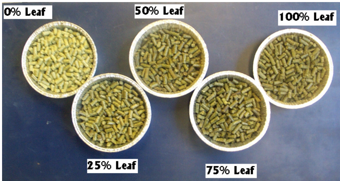
Figure 3. Photograph showing the color of fractionated alfalfa pellets with change in leaf content.
