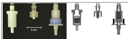
FIGURE 1. Photo and X-Ray of IX Cartridges (L-R, Alltech IC-OH, ORTG, Waters QMA)
