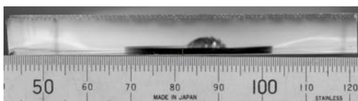
FIGURE 13. Top view of the irradiated glass plates after image processing for beam depth measurement, glass thickness = 10.05 mm.
