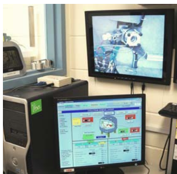
FIGURE 6. View of the solid target from the CCD camera during irradiation.
