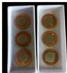
Figure 4. Mo-targets in alumina boats
