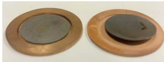
Figure 3. On the left a flat molybdenum plate versus the right, which contains a curved, sintered molybdenum plate.
