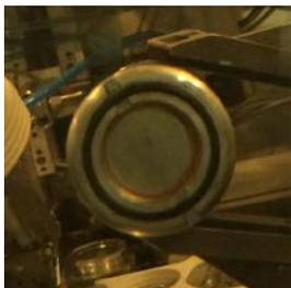
Figure 2. Enriched molybdenum target in capsule after irradiation on the GE PETtrace cyclotron.
