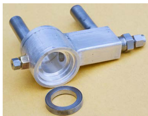
FIGURE 3. Cast silver target body and hardened stainless knife-edge-ring before pressing
