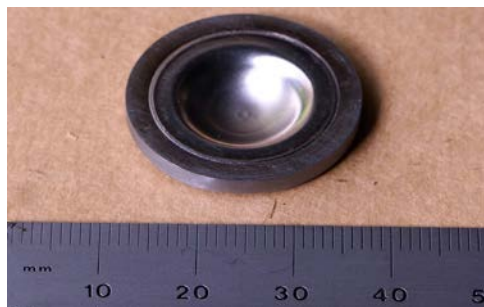
FIGURE 1. Electron-beam welded window module
