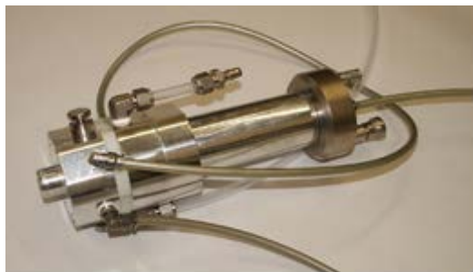
FIGURE 1. Gas target for ^{83}\text{Rb} production
