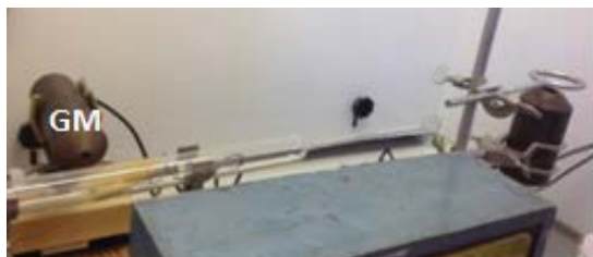
FIGURE 2. Detection system setup used in the Mo/Tc separation
