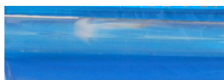
FIGURE 6. \text{MoO}_3 crystals deposited in a white – yellowish layer on the quartz tube walls
