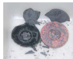
FIGURE 5. Copper target support after the separation of Mo/Tc generated in situ by irradiation of disc Mo targets with 15 MeV proton beam at 50 \mu\text{A} . \text{CuO} (black)
