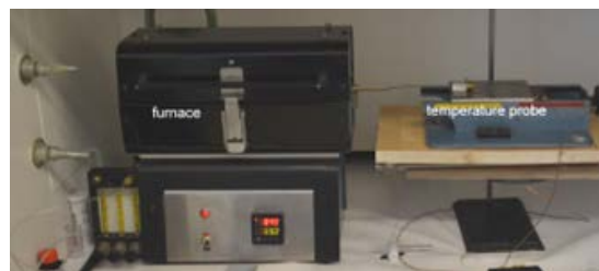
FIGURE 1. Experimental system used in the \text{Mo}/^{99m}\text{Tc} thermal separation experiments
