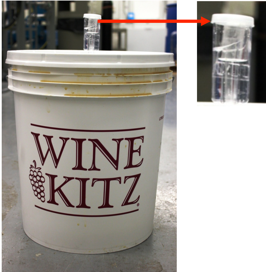
Figure 4.2 25 L wine pail equipped with a gas trap
