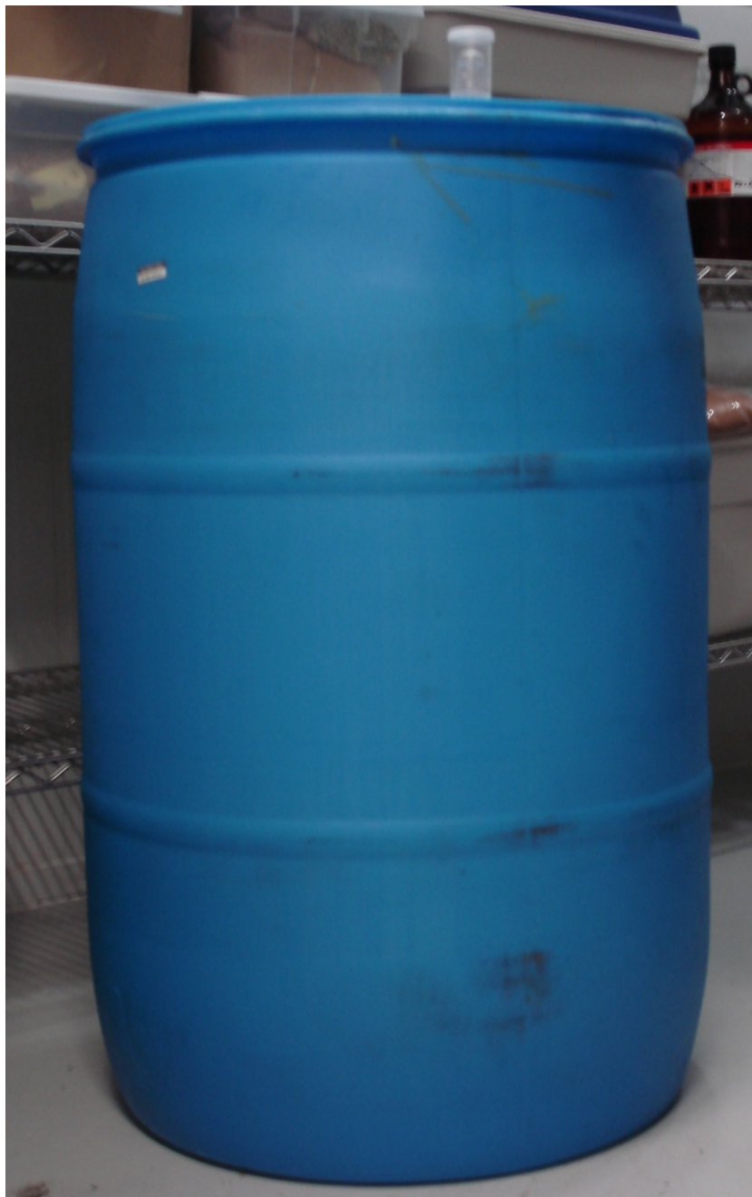
Figure 4.3 210 L polyethylene drum equipped with a gas trap
