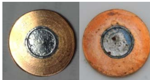
FIGURE 4. Circular 100 Mo target before (left) and after (right) irradiation for 1 h with 15 MeV protons at 50 μA
