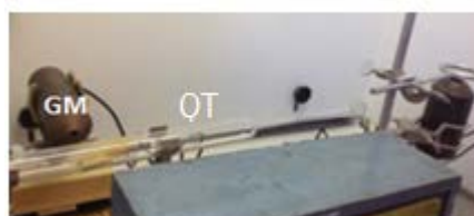
FIGURE 3. Apparatus used to measure activity with a Geiger Muller (GM) tube along the length of the quartz tube (QT) after Mo/Tc separation.
