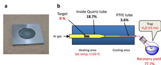
FIGURE 1. a)  $\text{Cu}_2\text{Se}$  target put in a tungsten backing; b) Illustration of optimized dry-distillation apparatus and distribution of radioactivity
